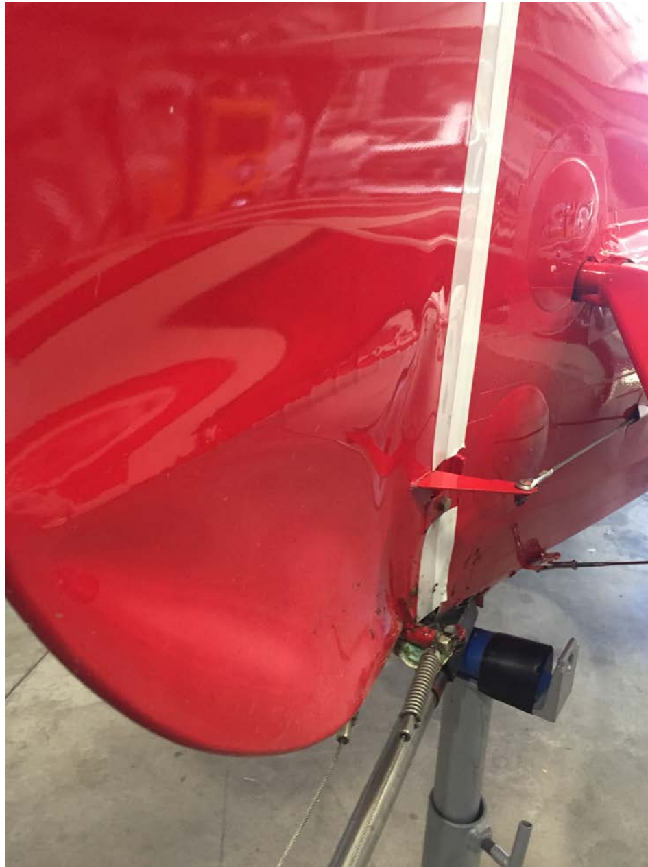
Photo 2 - View of rudder damage (photo courtesy of the FAA)
