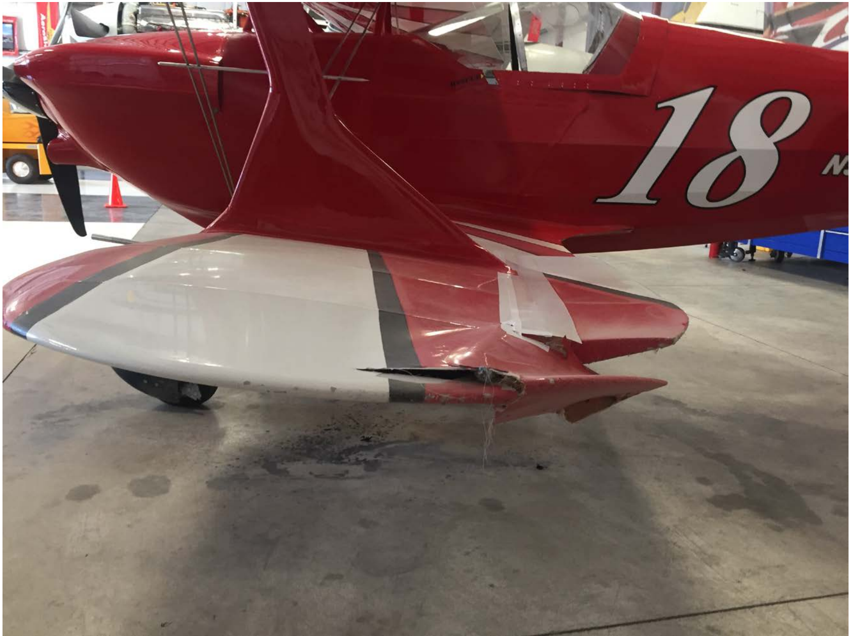
Photo 1 – View of lower left wing damage (photo courtesy of the FAA)
