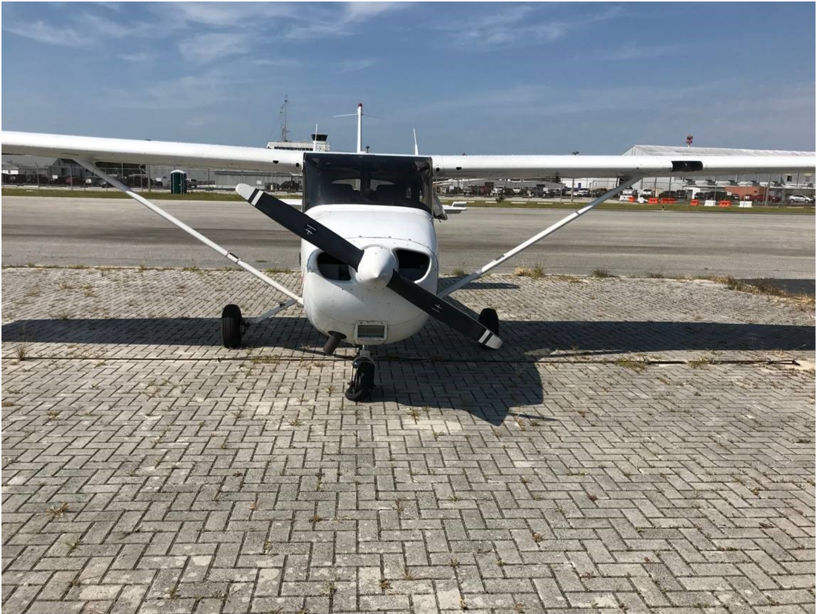
Photo 1 – View of flat nose wheel (photo courtesy of the FAA)
