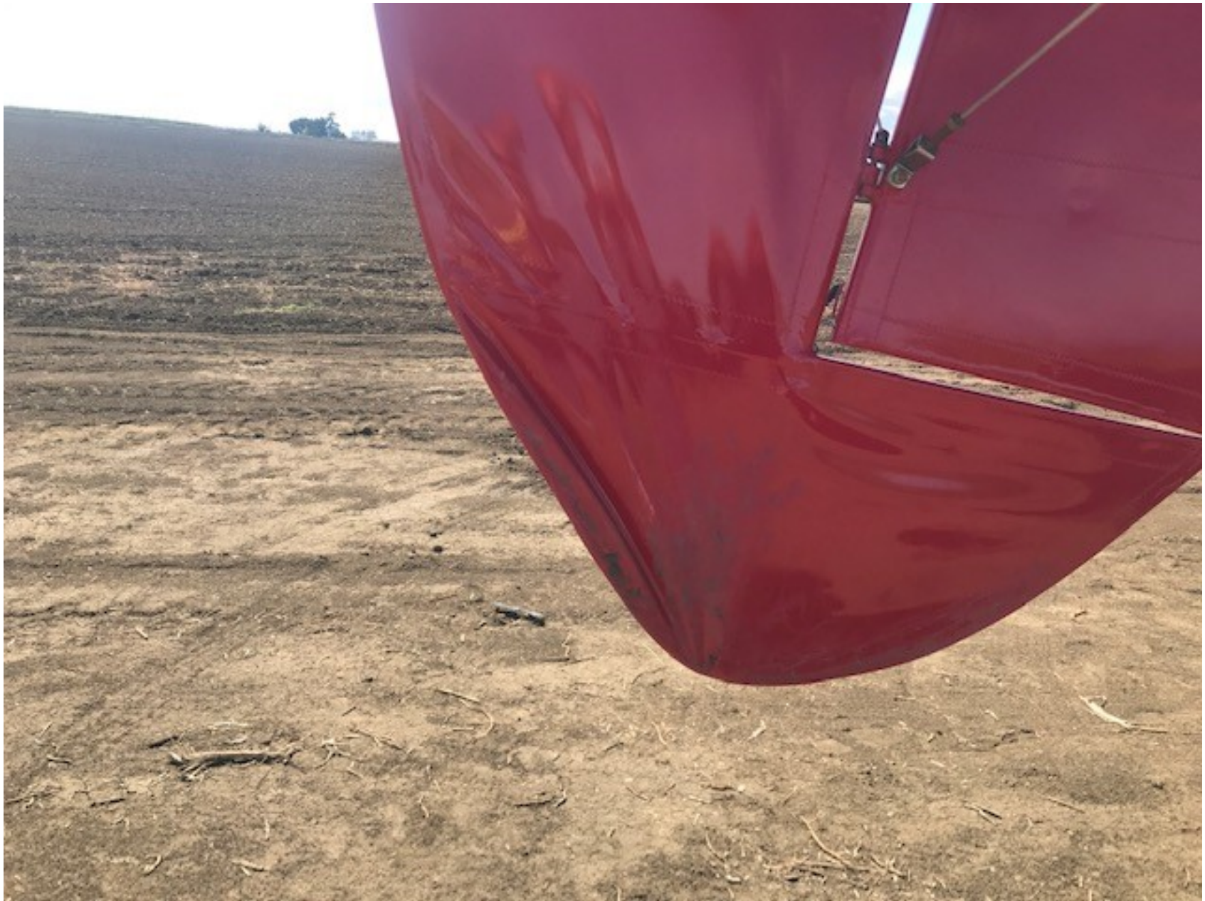
Photo 3 - View of rudder damage (photo courtesy of the pilot)
