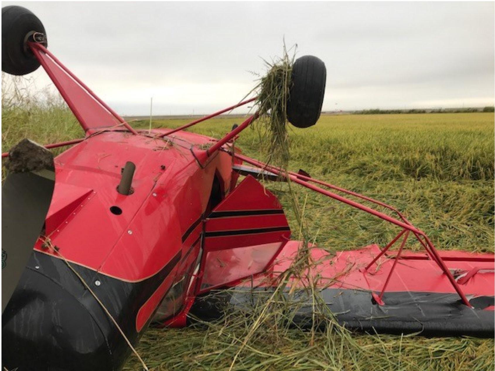
Photo 2 - View of right wing lift strut damage (photo courtesy of the pilot)
