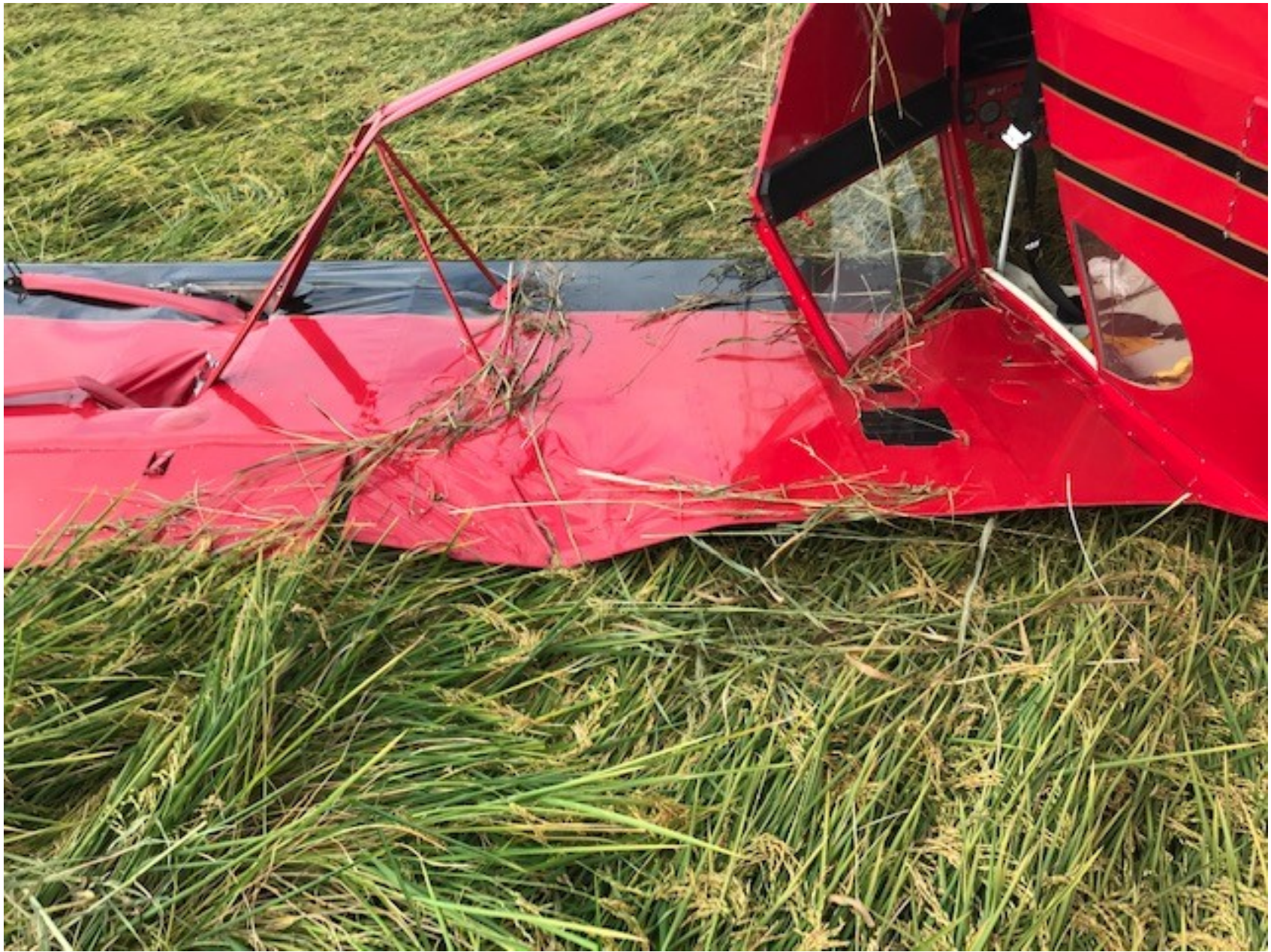
Photo 4 - View of right wing damage (photo courtesy of the pilot)
