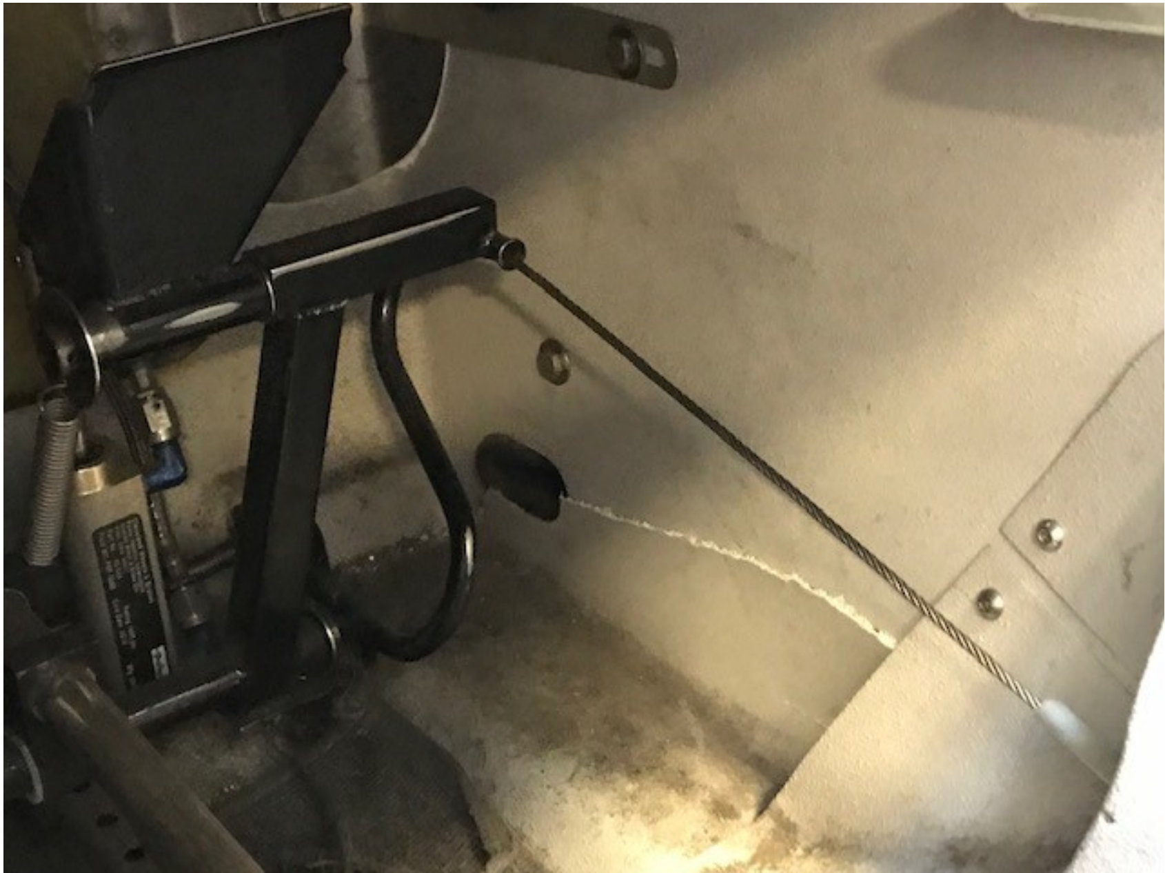
Photo 2 – View of damaged floor board (courtesy of the FAA)
