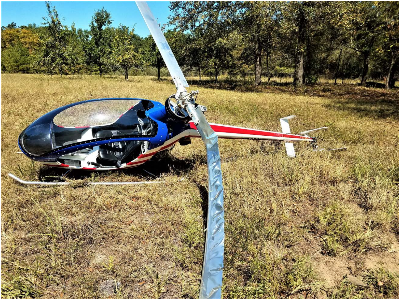
Photo 1 – View of damaged main rotor blades (courtesy of the pilot)
