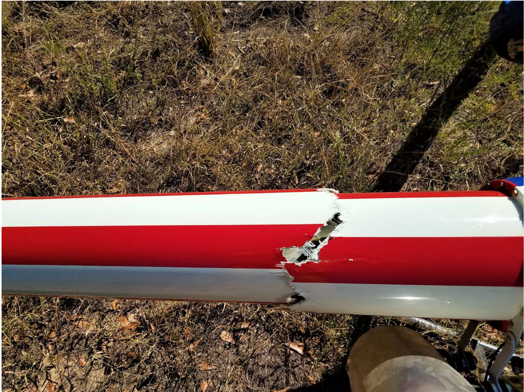
Photo 2 – View of damaged tailboom (courtesy of the pilot)
