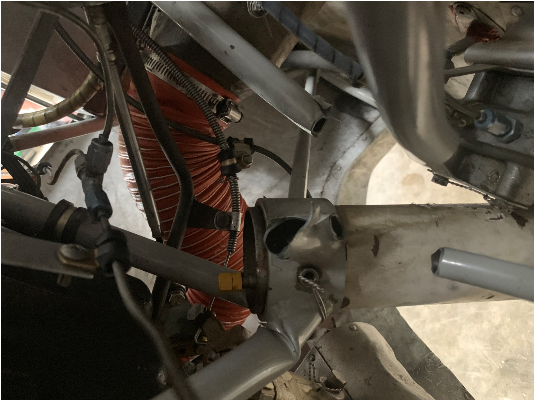
Photo 1 – View of damaged engine mount (Photo courtesy of the FAA)
