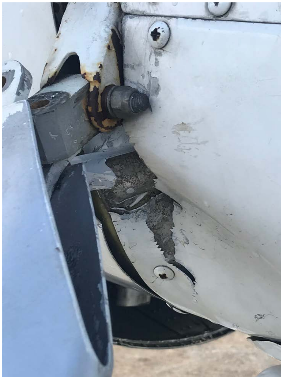
Photo – View of damage to fuselage and float attachment point (Courtesy of the FAA)
