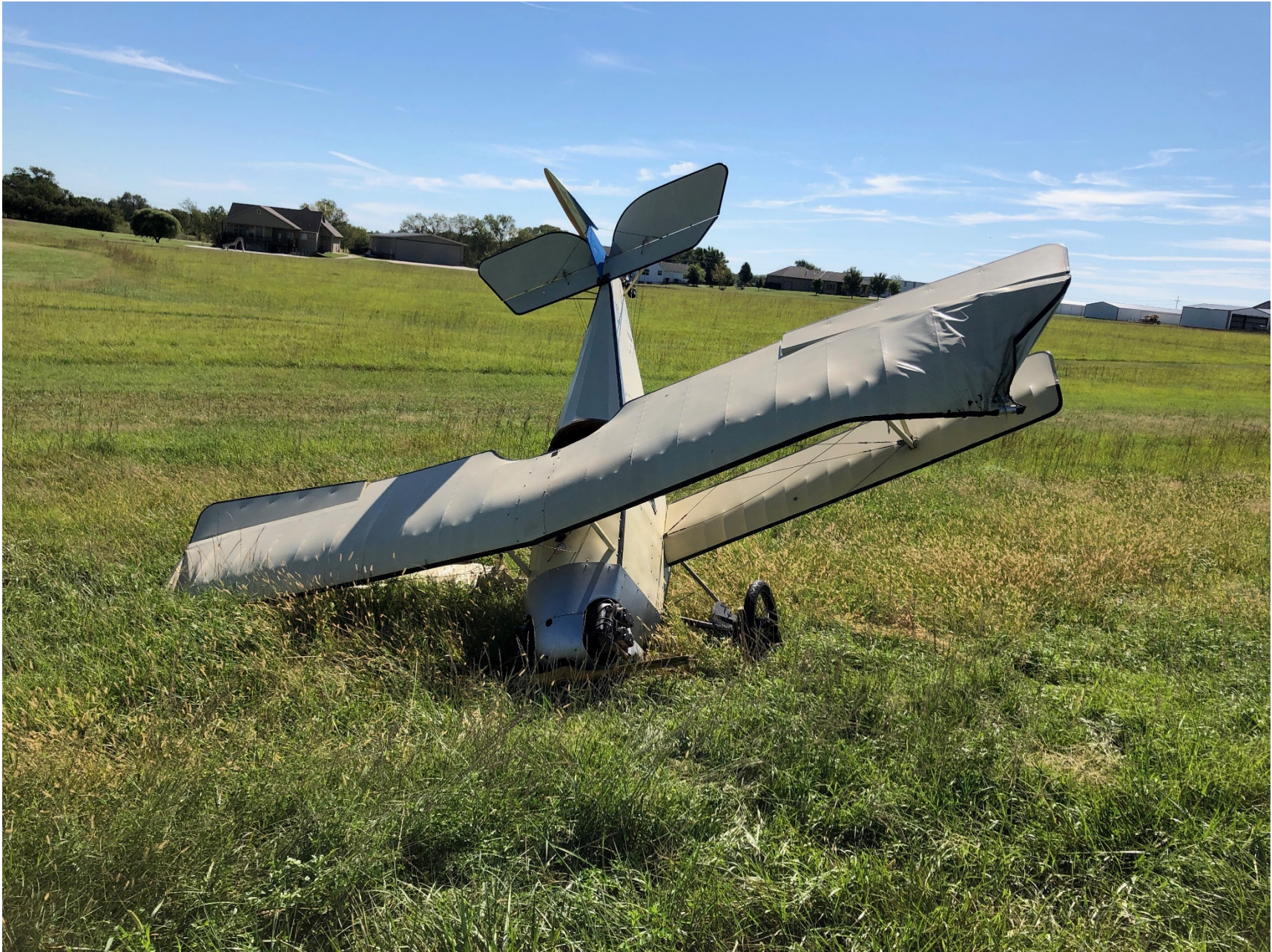
Photo 1 – View of damaged lower right and upper left wing (Photo courtesy of the FAA)
