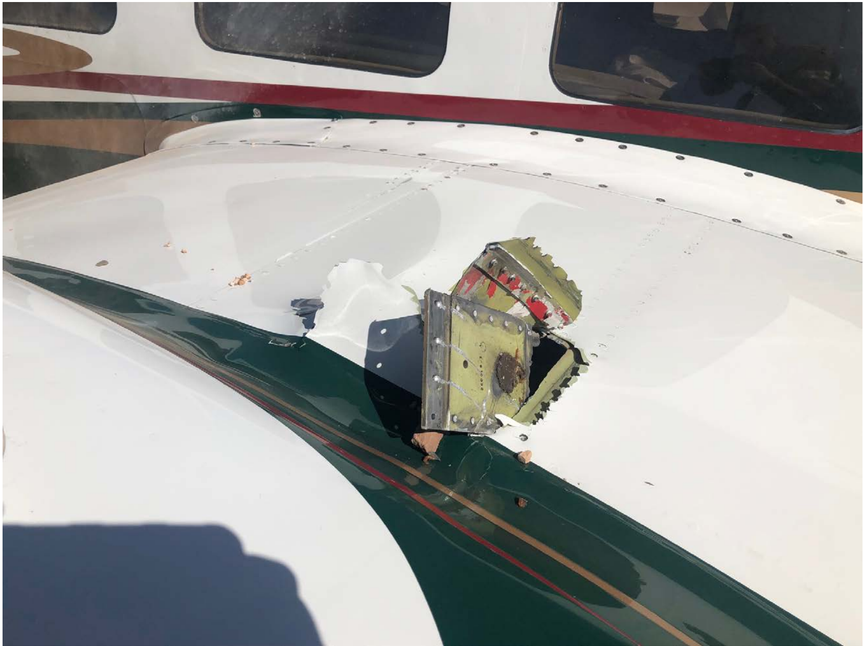
Photo 2 - View of right wing damage (photo courtesy of the pilot)
