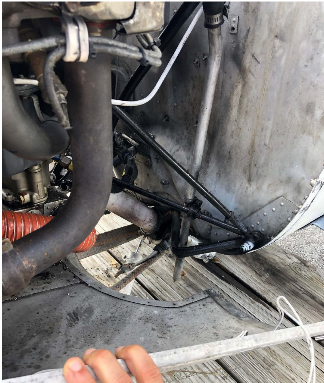
Photo 1 – View of damaged engine mount (Photo courtesy of the operator)
