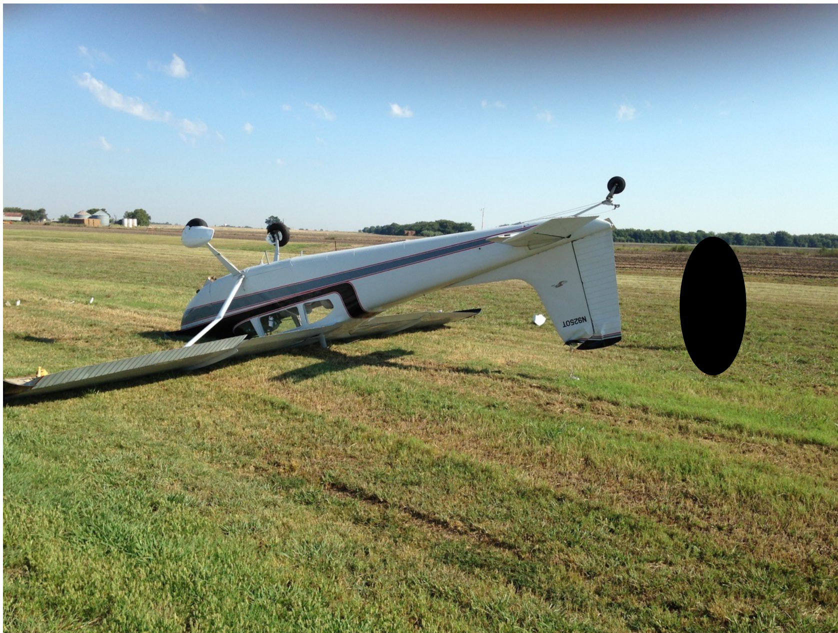
Photo 1 – View of damaged right-wing lift strut and empennage (courtesy of the FAA)
