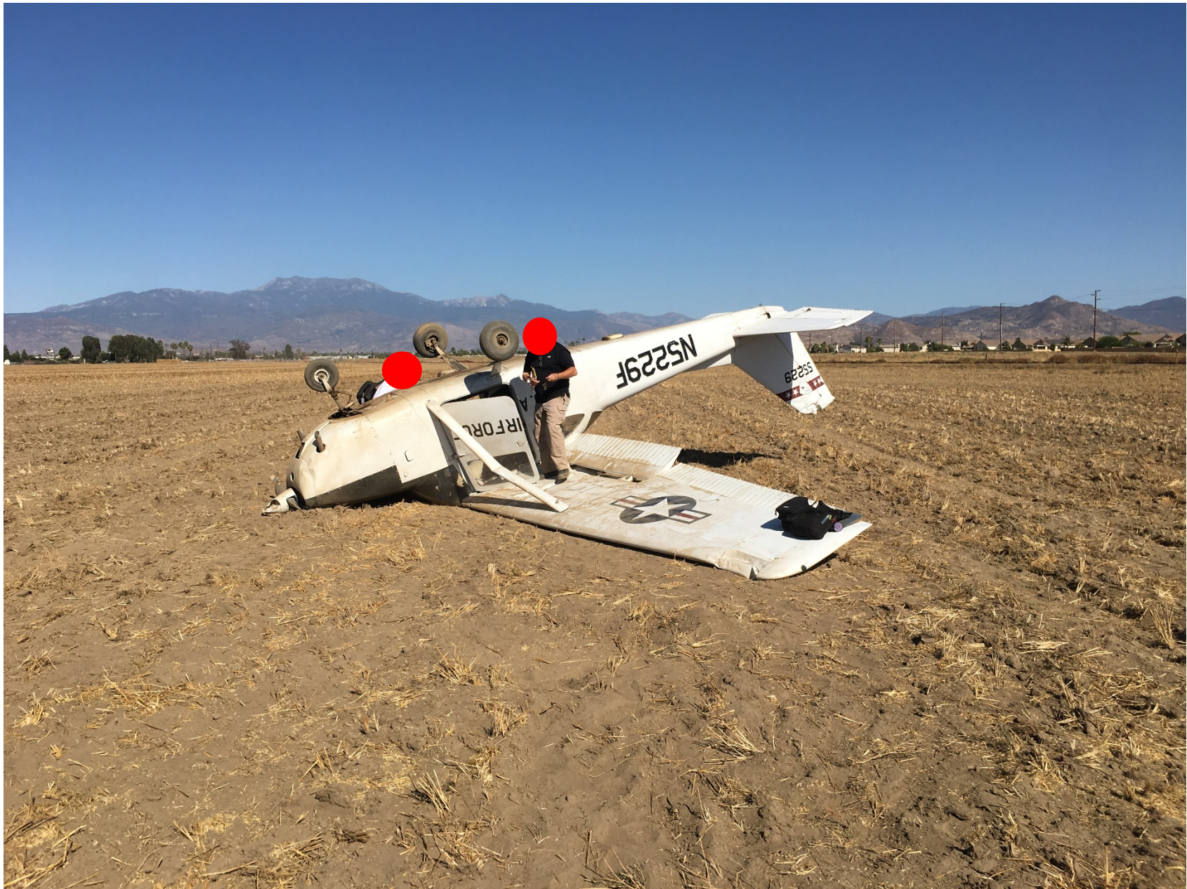
Photo 1 – View of damaged right-wing lift strut and vertical stabilizer (courtesy of the pilot)
