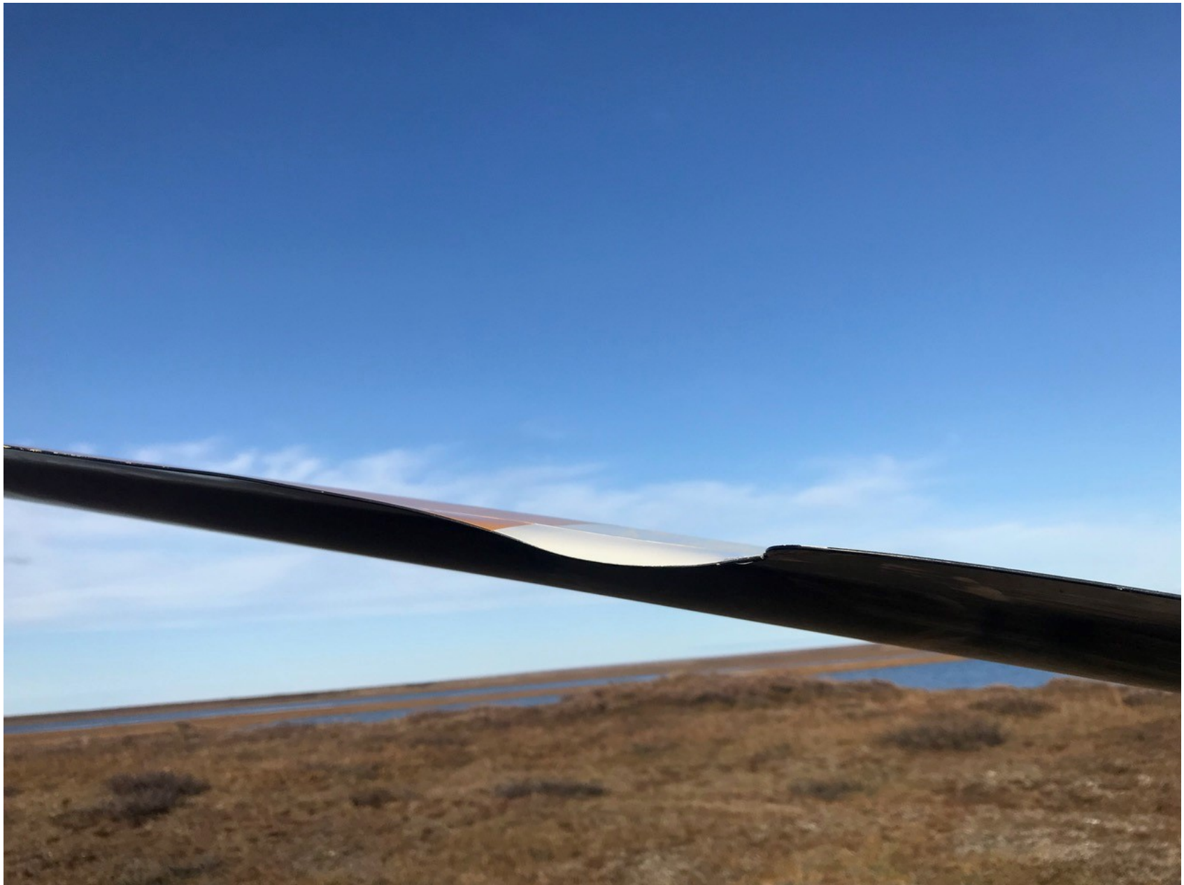
Photo 1 – View of damage sustained to main rotor blade (Courtesy of FAA)
