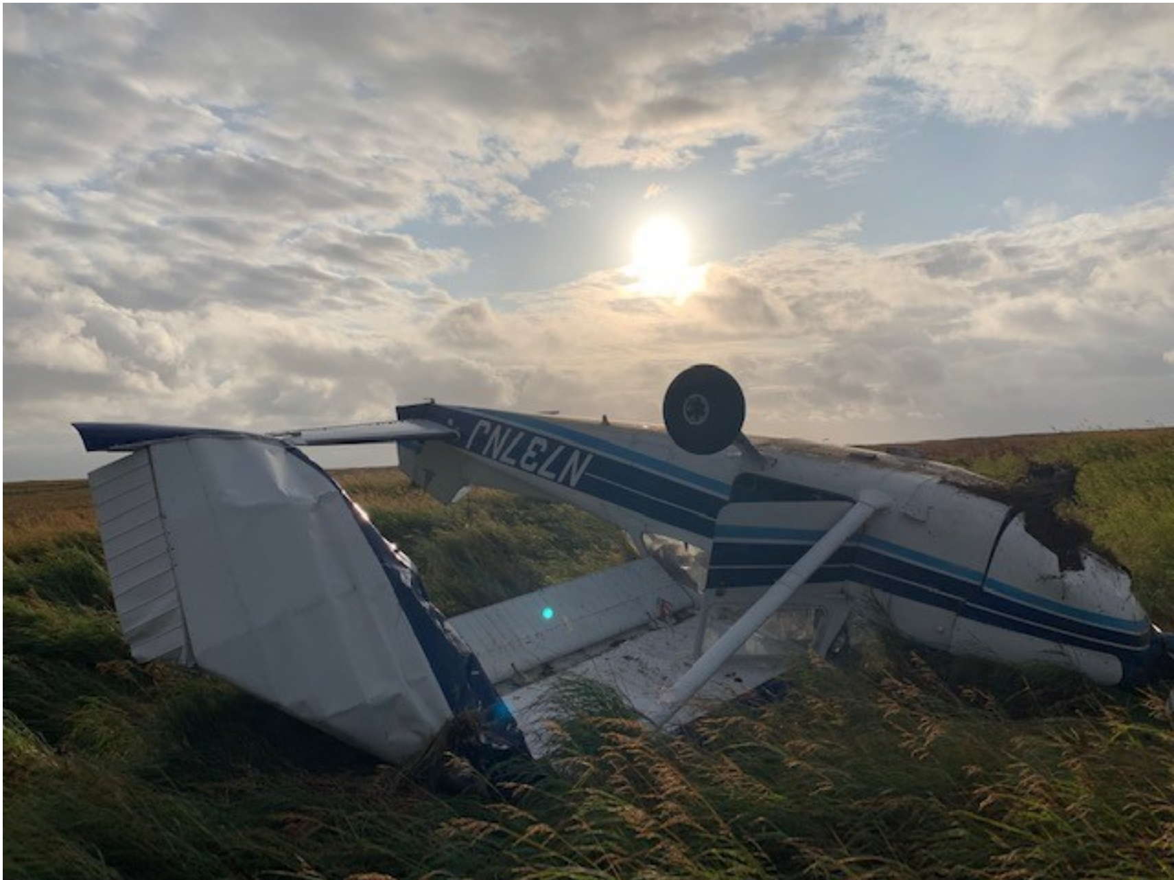
Photo 1 – View of inverted airplane with damaged left wing (Photo courtesy of the pilot)
