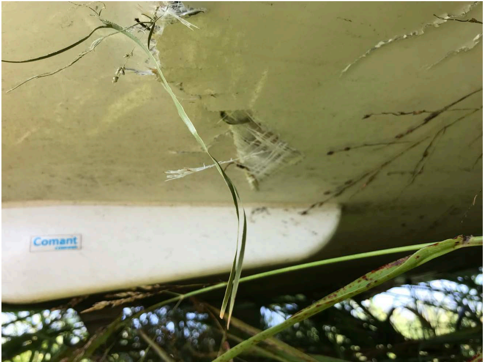
Photo 1 – View of damage to the composite lower fuselage (Courtesy of FAA)
