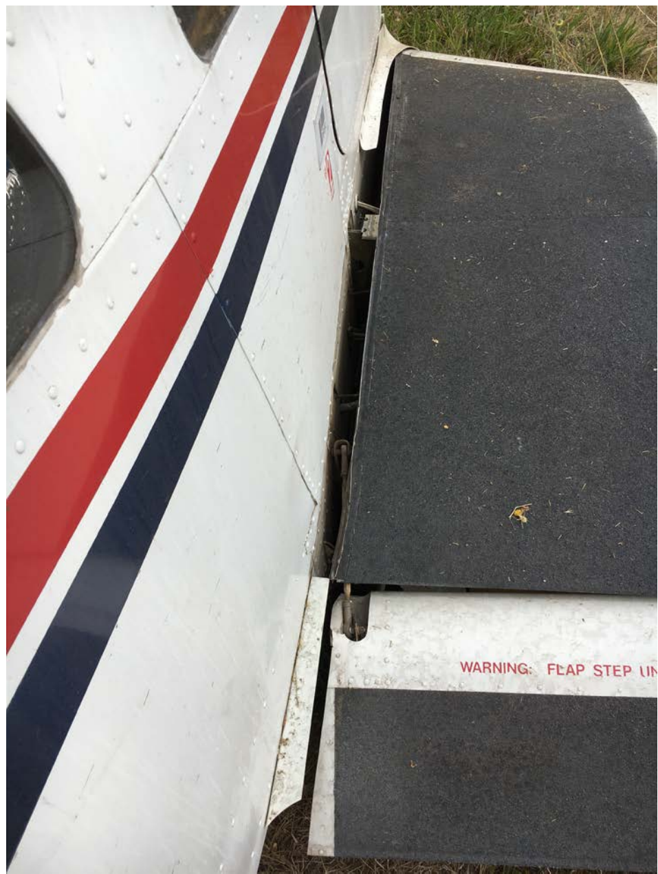
Photo 2 – View of separated right-wing root (courtesy of the FAA)
