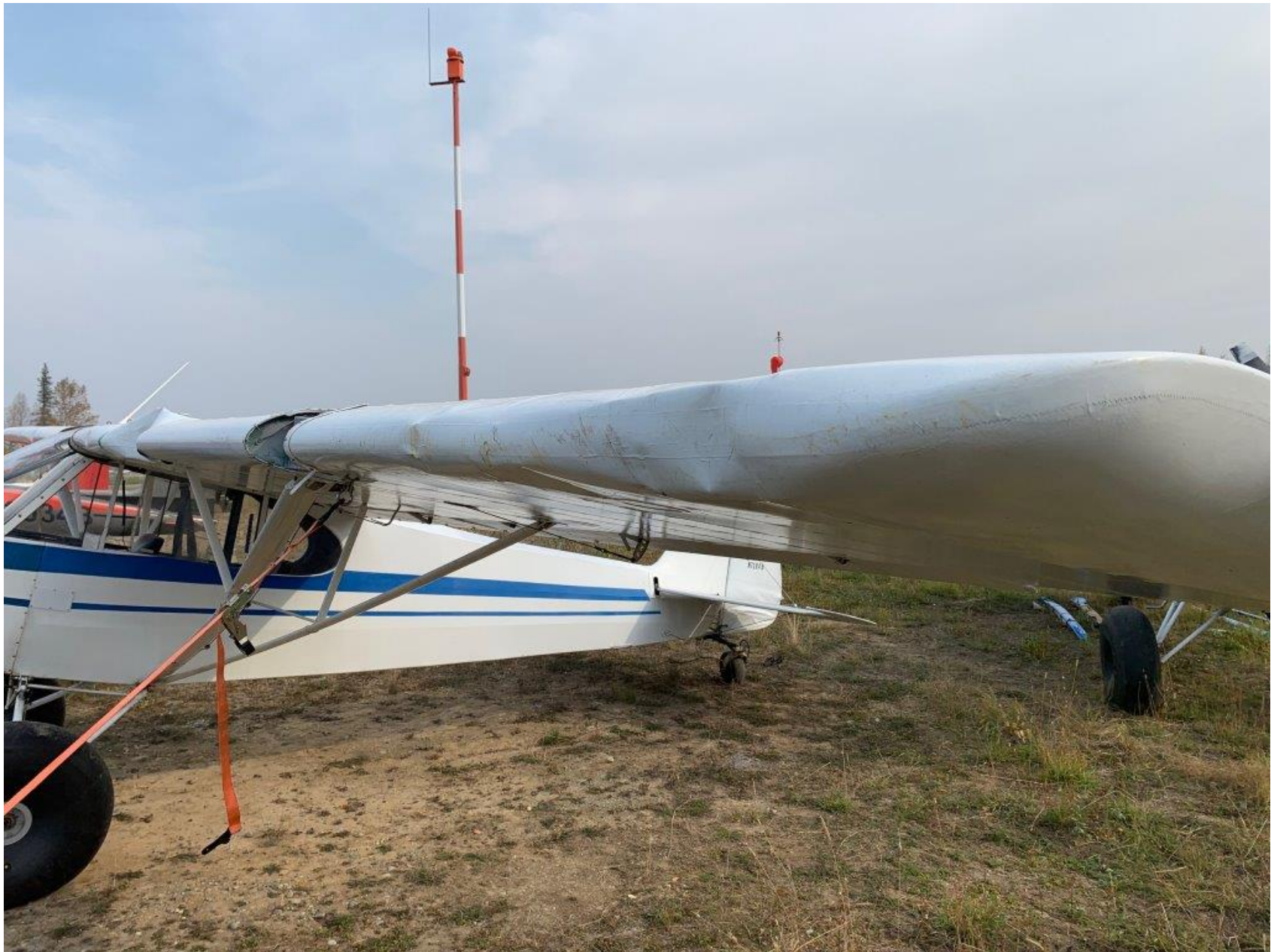
Photo 1 – View of the left wing damage (photo courtesy of the pilot)
