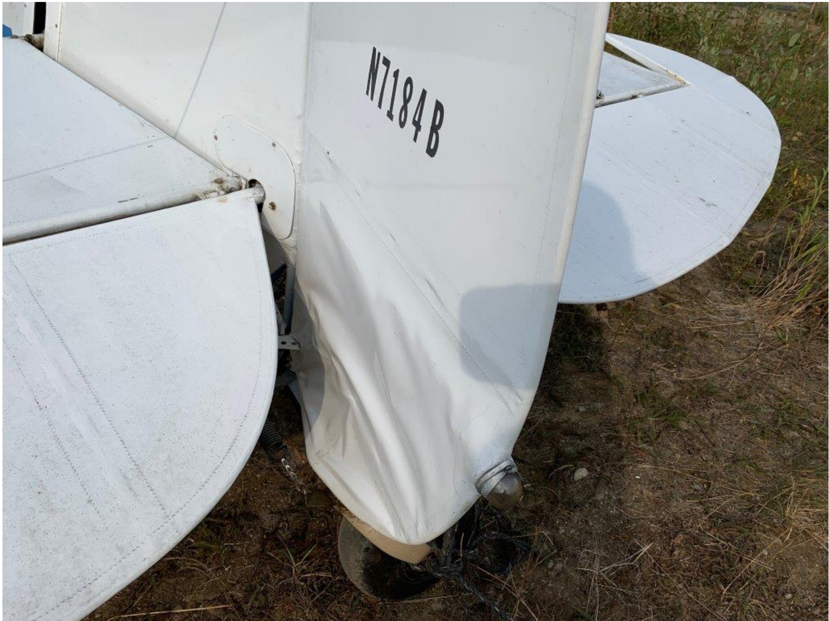
Photo 2 - View of rudder damage (photo courtesy of the pilot)
