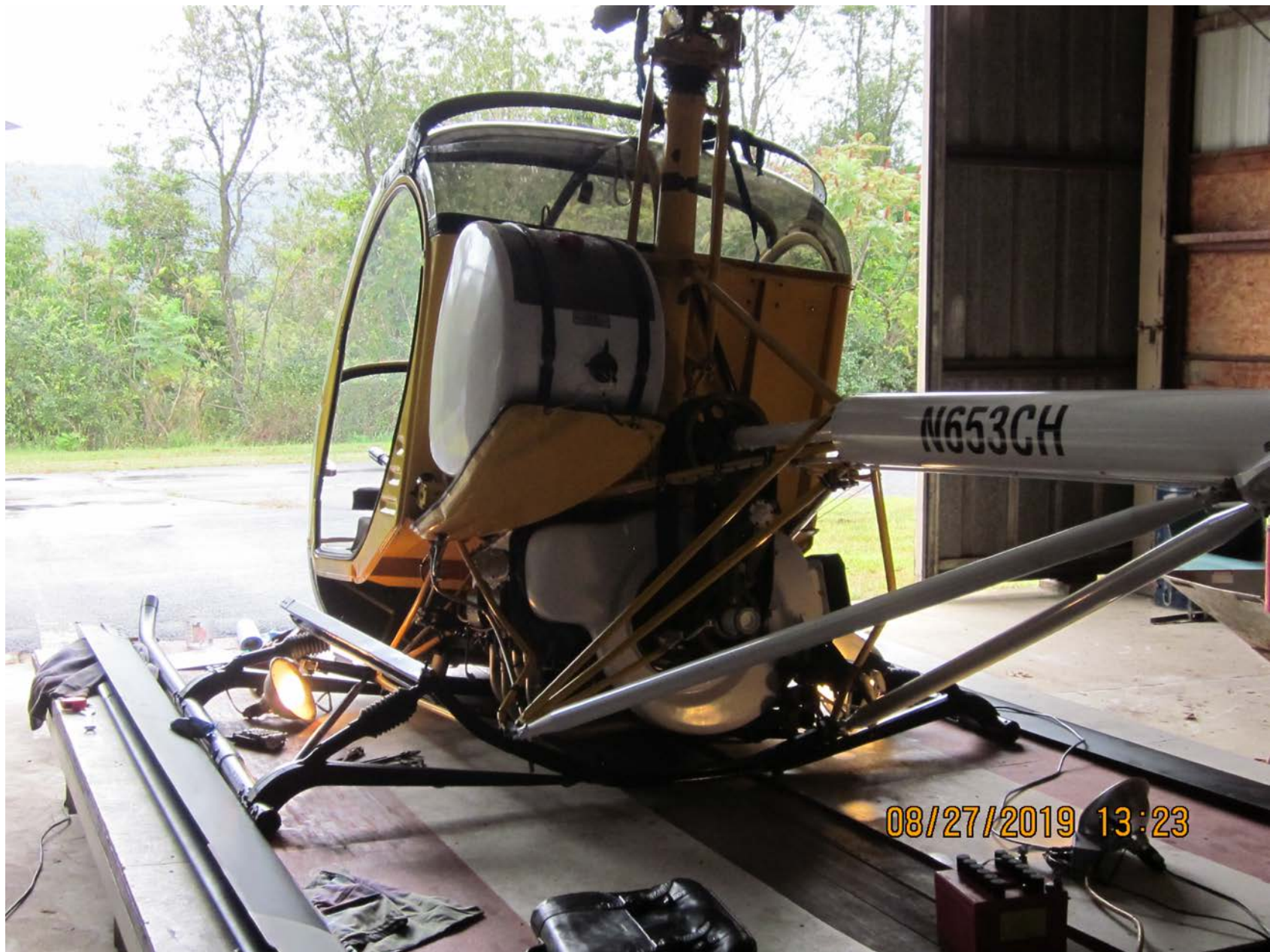
Photo 1 – View of damage to the aft crossmember (Courtesy of Operator)
