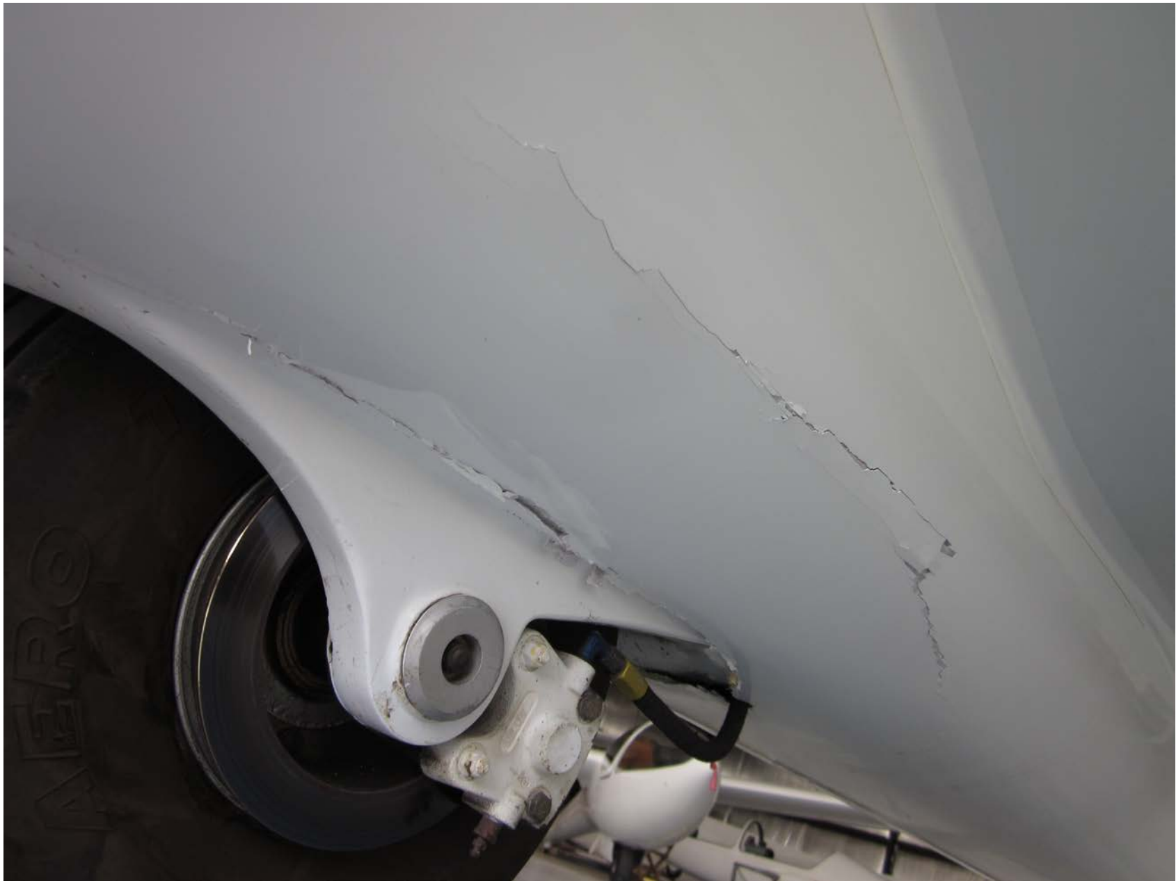
Photo 2 – View of damage to the composite structure of the lower fuselage (Courtesy of FAA)
