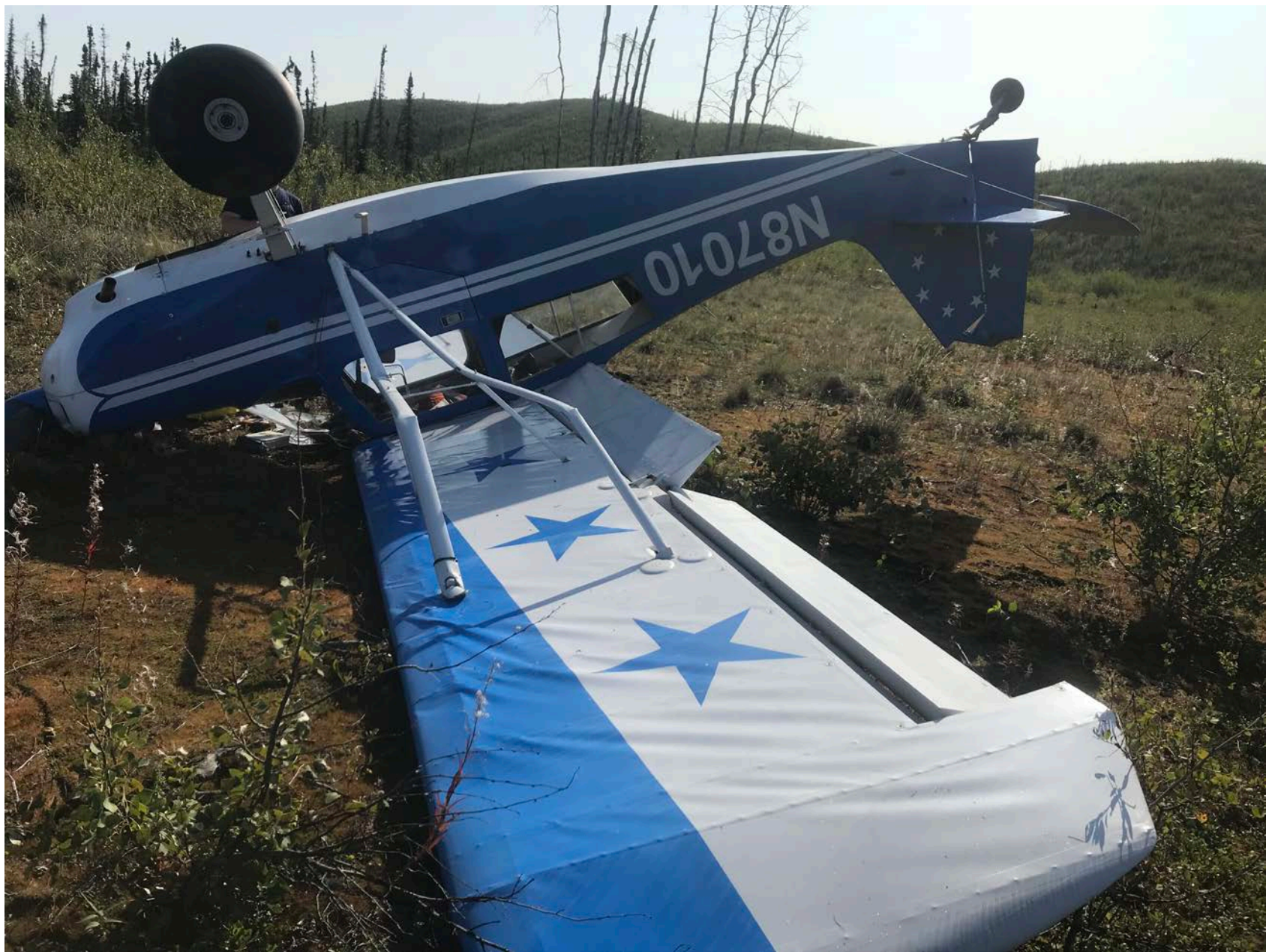
Photo 1 – View of damaged right wing lift struts (courtesy of the pilot)
