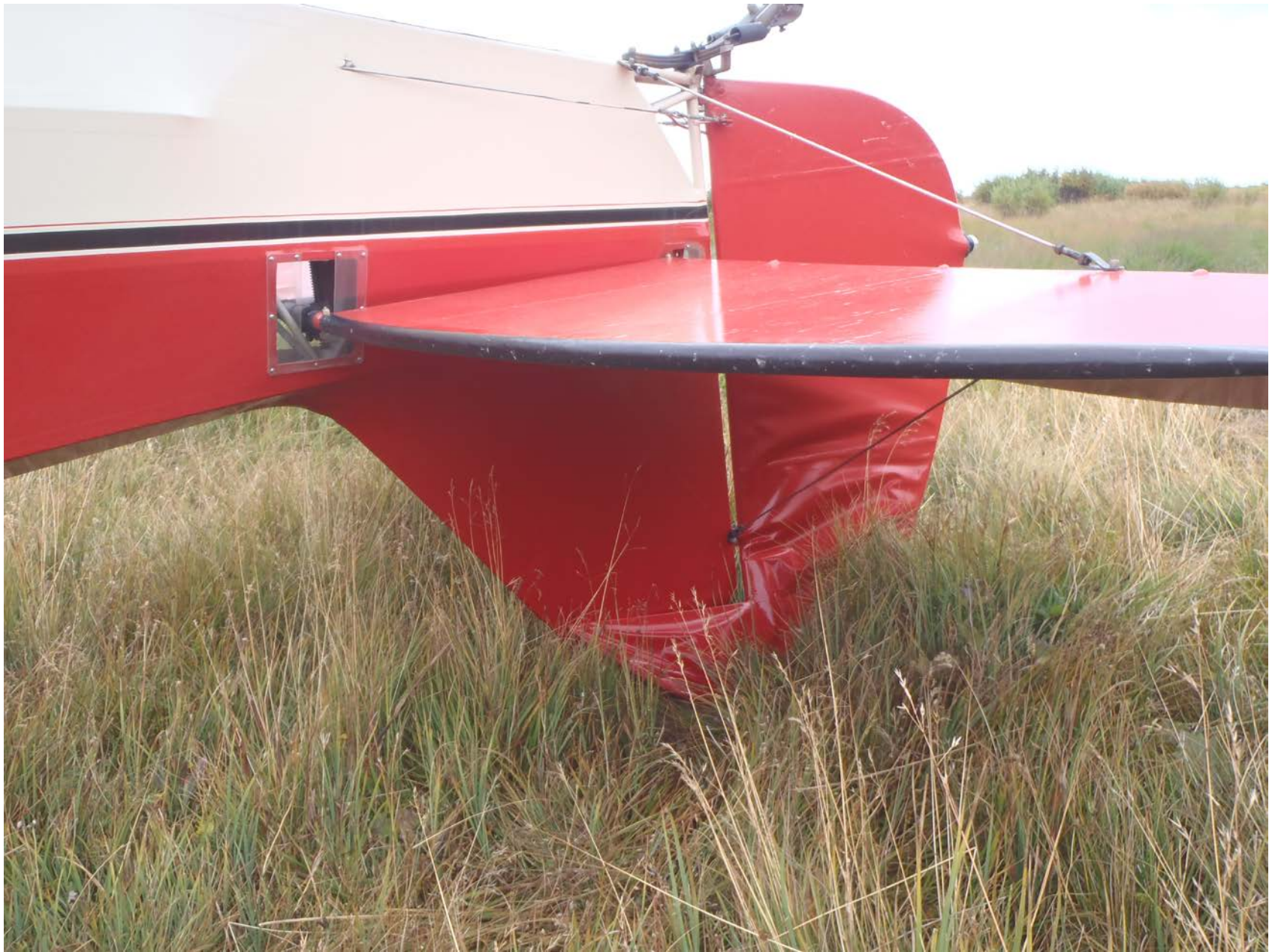
Photo 1 – View of damaged empennage (courtesy of the pilot)
