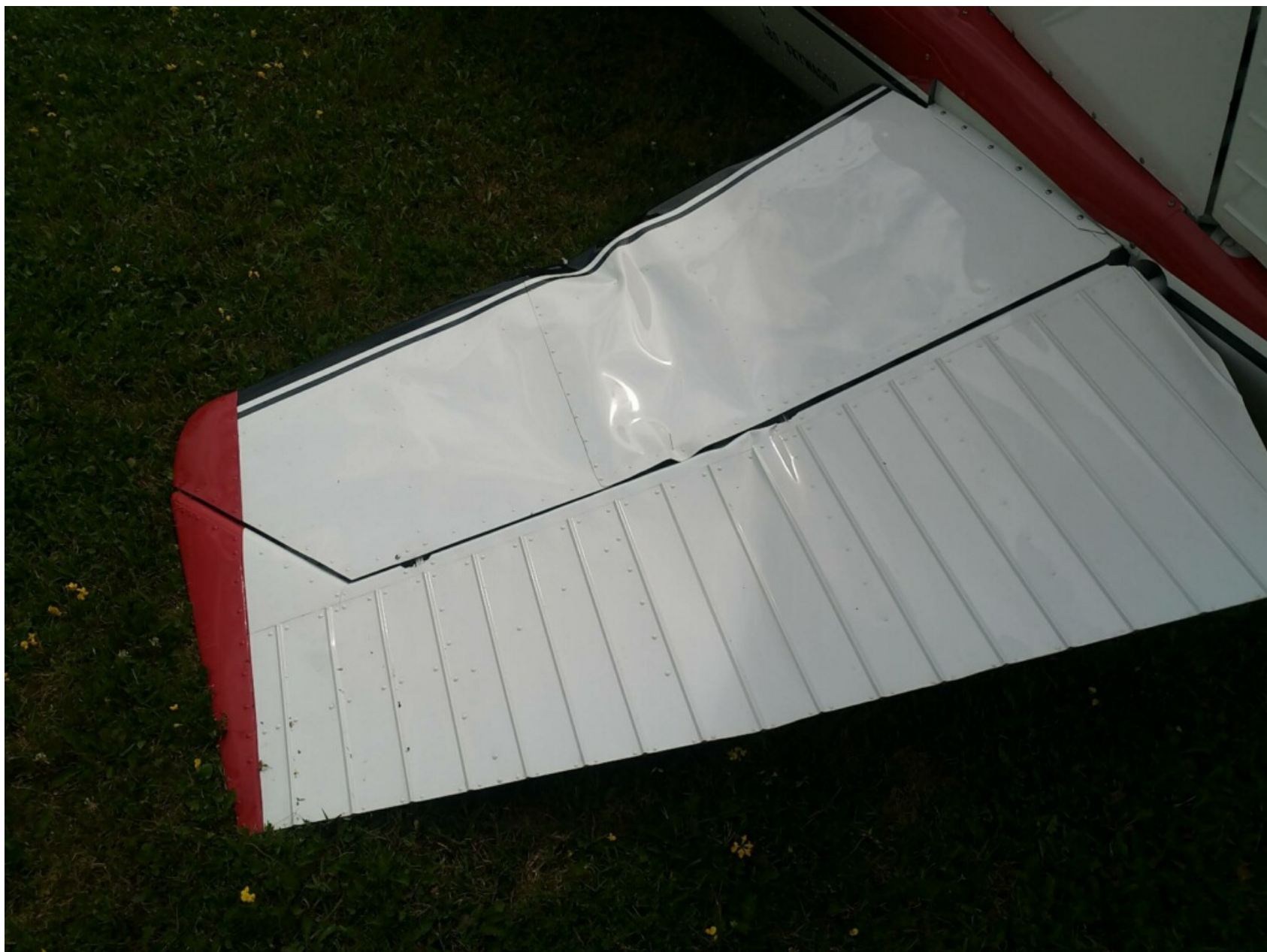
Photo 2 – View of damaged left horizontal stabilizer (courtesy of the pilot)
