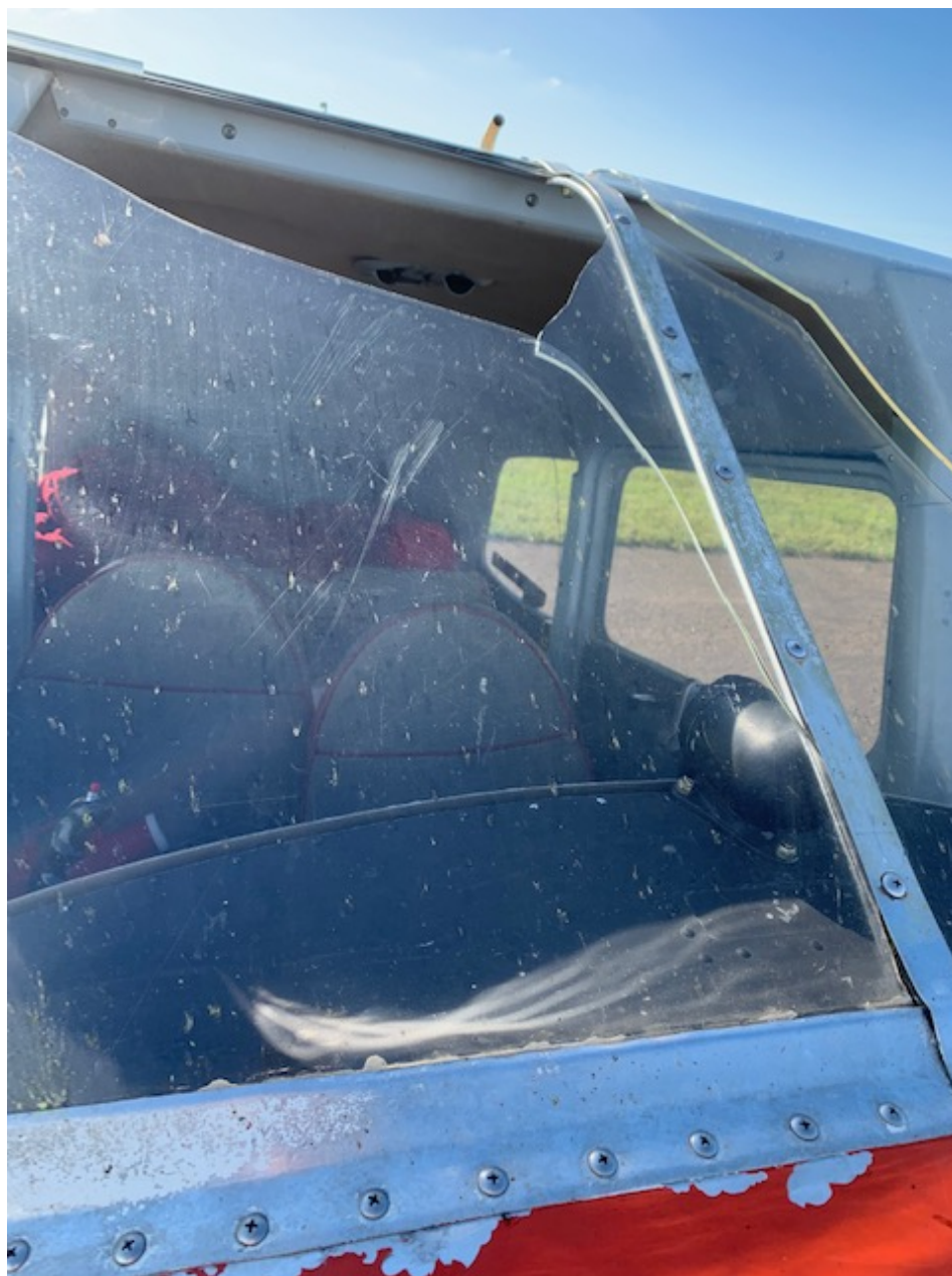
Photo 2 - View of windscreen damage (photo courtesy of the FAA)
