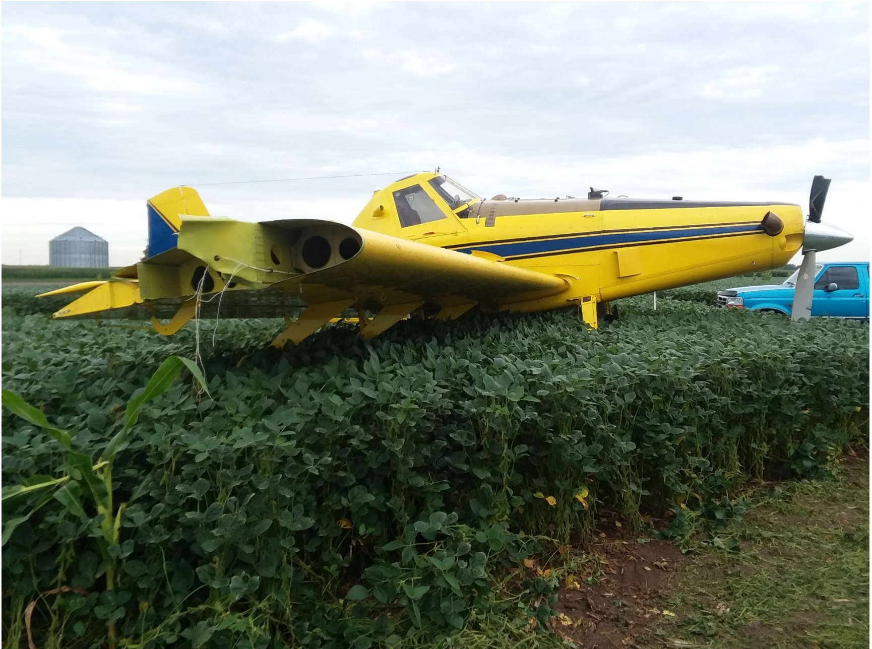
Photo 1 – View of damaged right wing of airplane in a bean field (Photo courtesy of the FAA)
