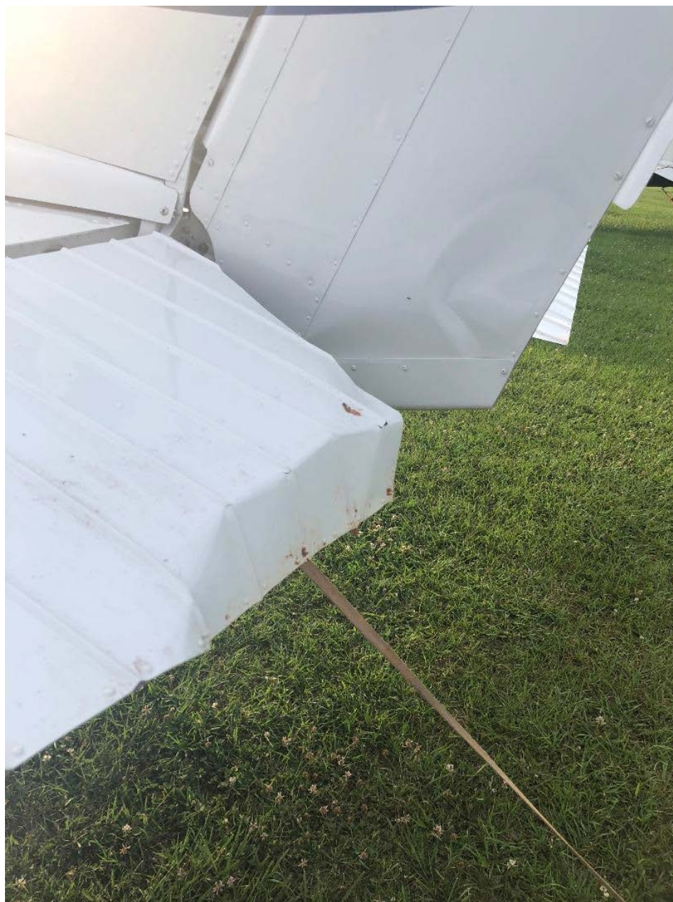
Photo 1 – View of damage to the rudder (Courtesy of FAA)
