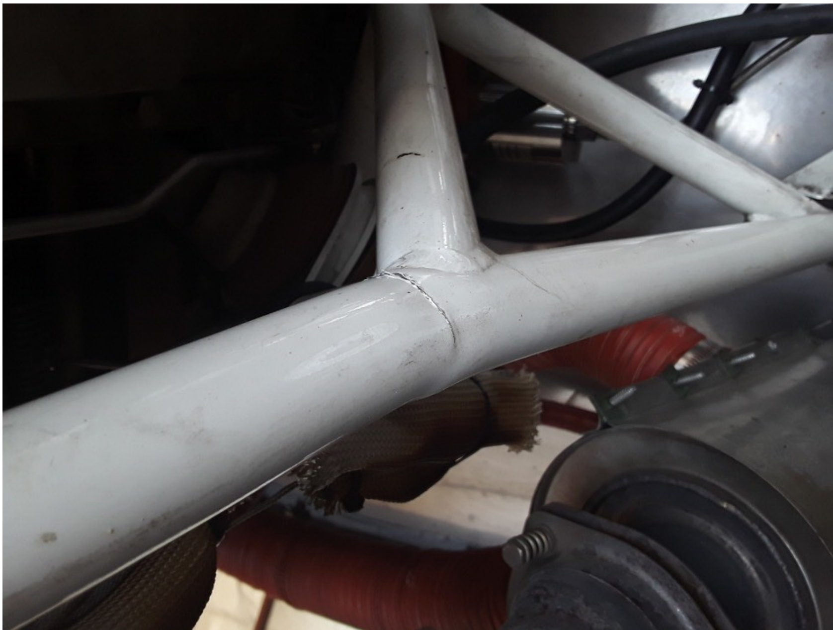
Photo 1 – View of engine mount damage (photo courtesy of the FAA)
