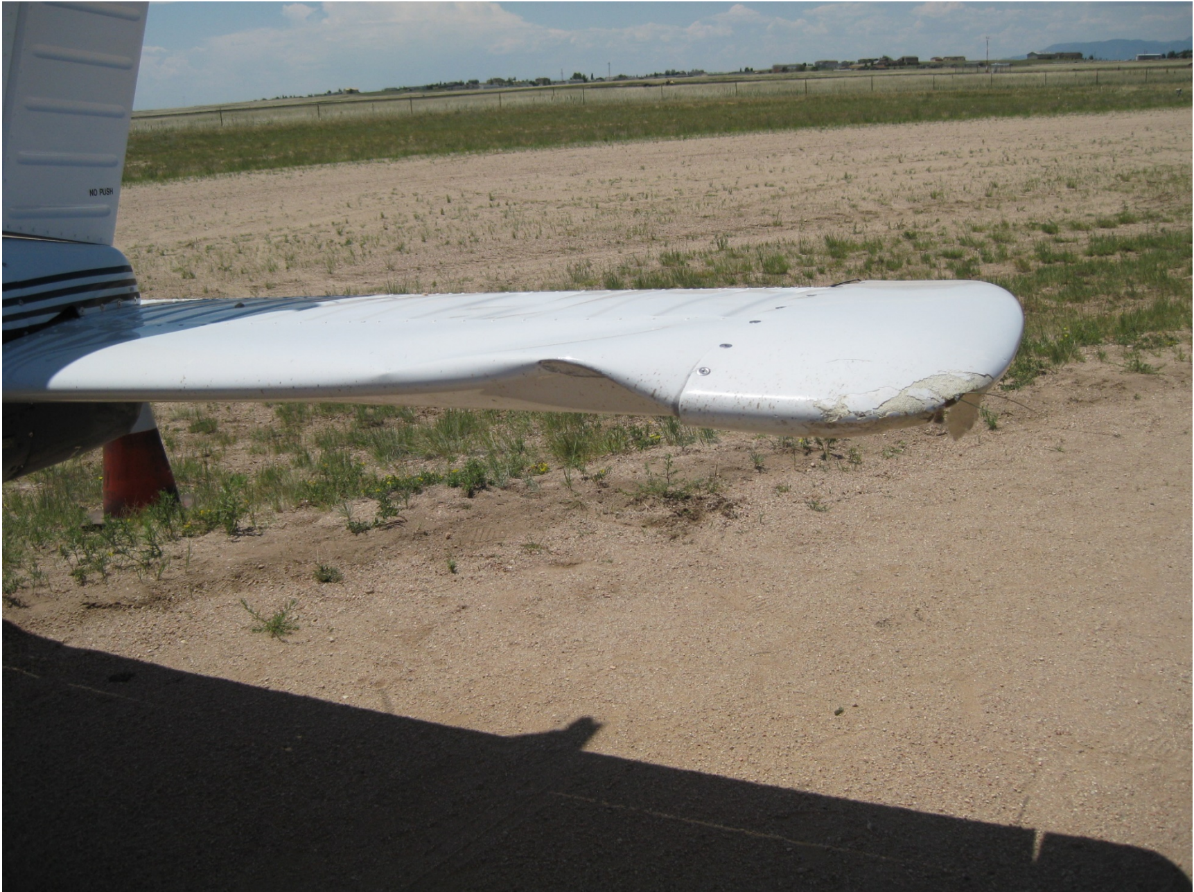
Photo 1 – View of damaged left stabilator (Photo courtesy of the FAA)
