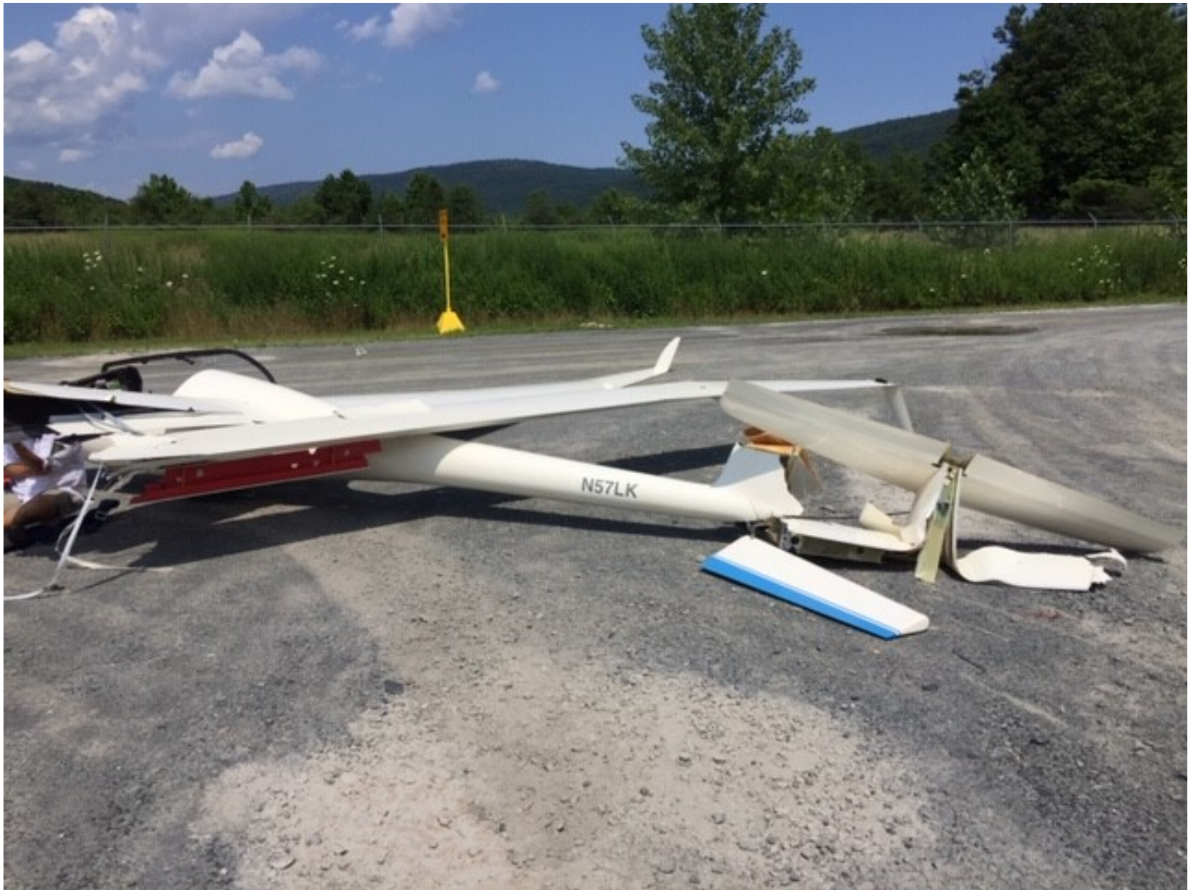
Photo 1 – View of damage to empennage (Courtesy of FAA)
