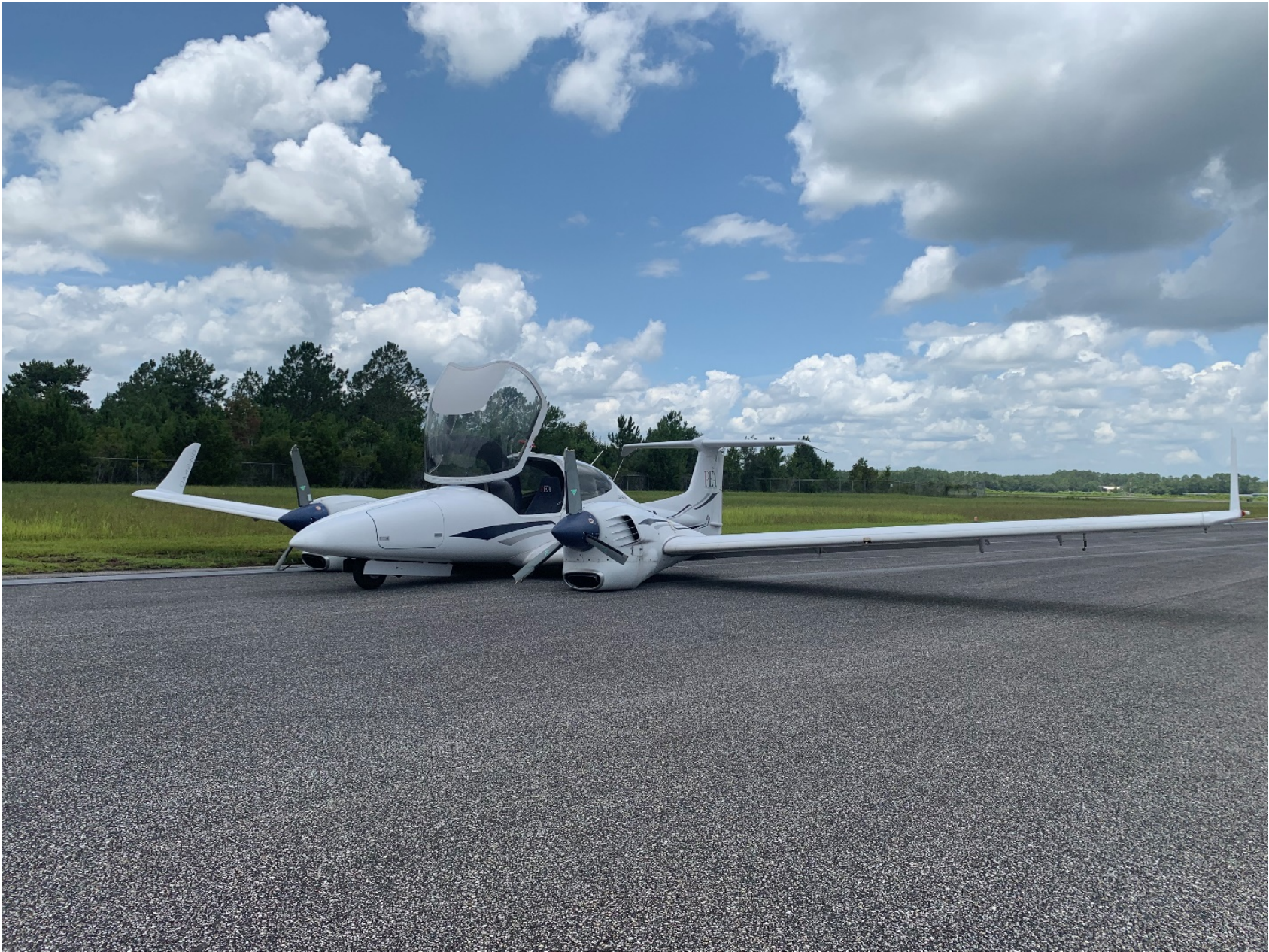
Photo 1 – View of the airplane on the runway with the gear up (photo courtesy of the pilot)
