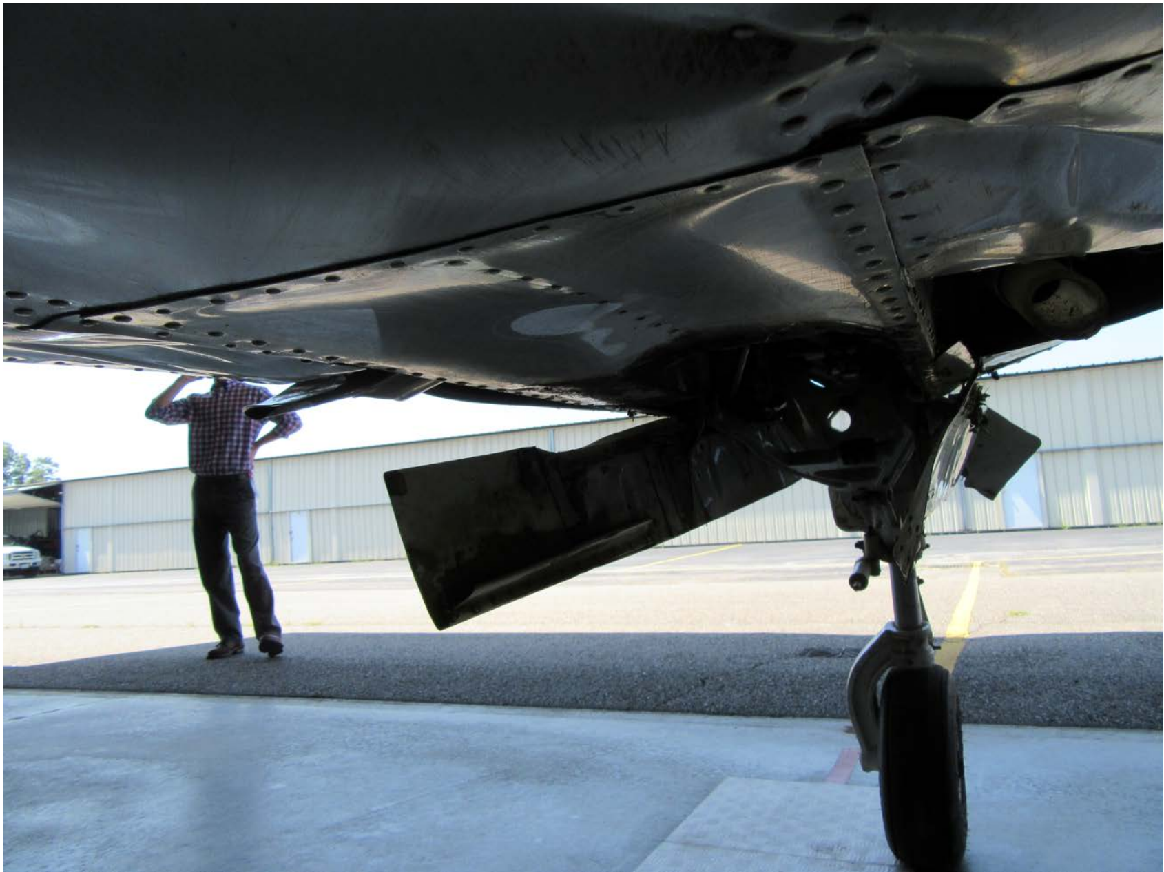
Photo 1 – View of damage to the lower fuselage (Courtesy of FAA)
