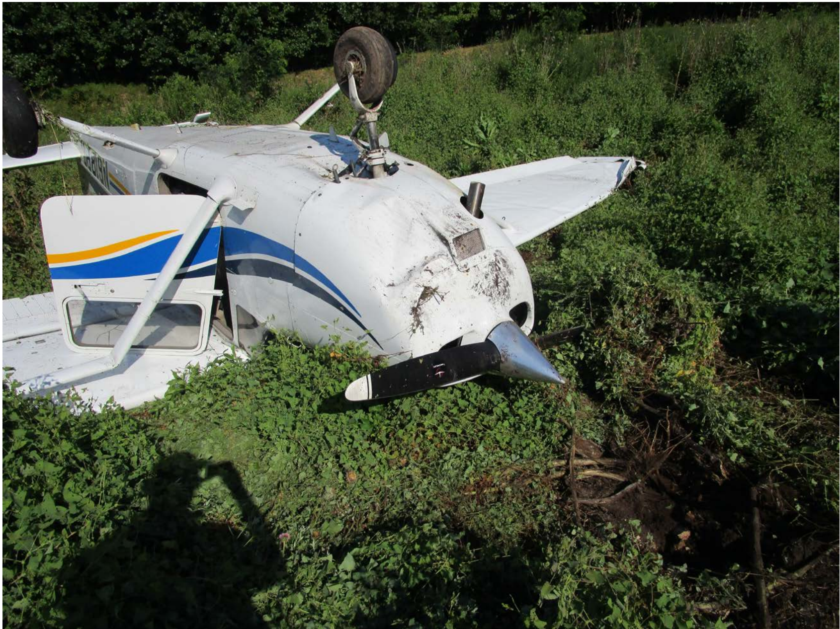
Photo 1 – View of nosed over airplane with damage to left wing lift strut (courtesy of the FAA)
