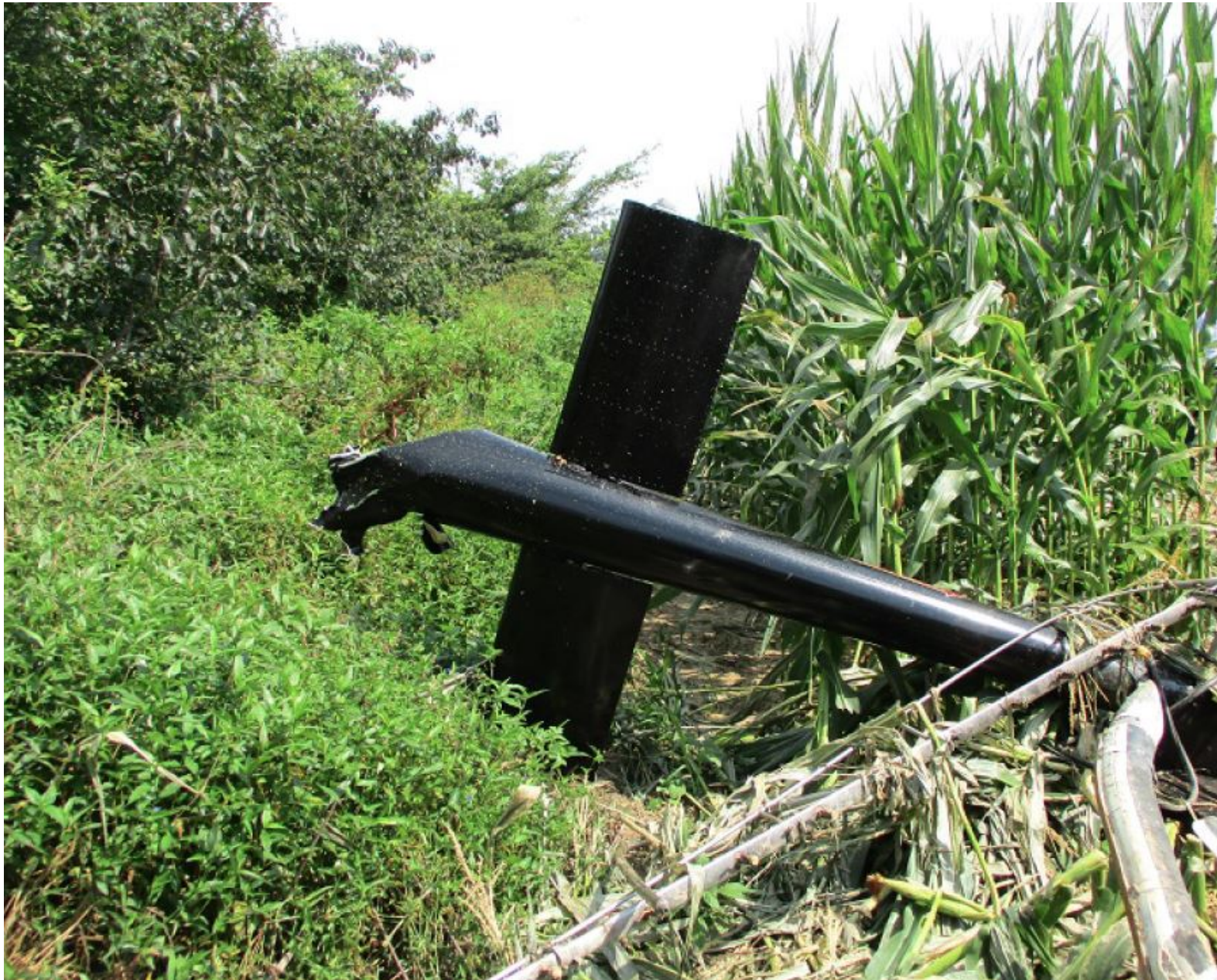
Photo 1 – View of damaged and separated tailcone (courtesy of the pilot)
