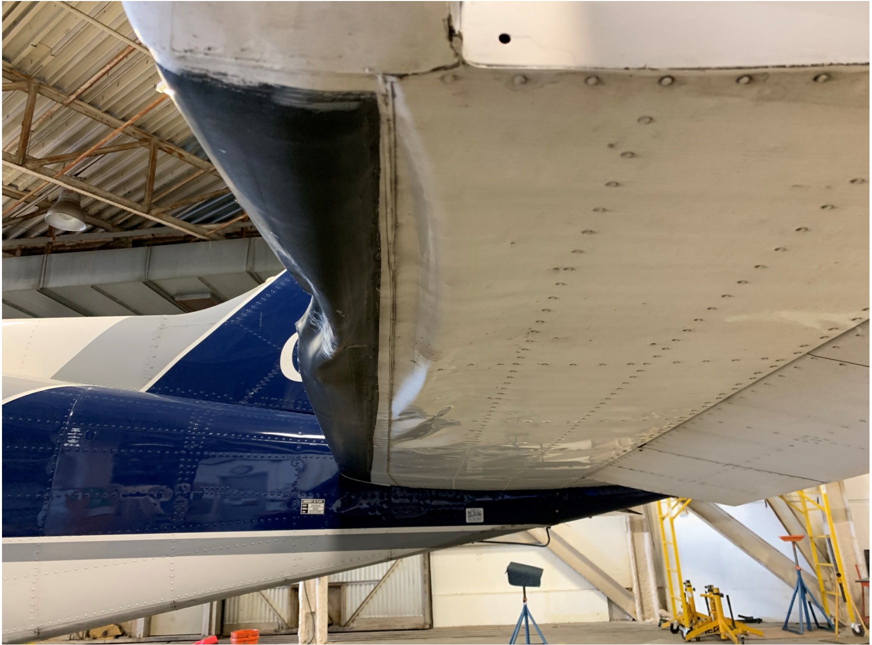
Photo 1 – View of left horizontal stabilizer damage from underneath (Photo courtesy of the operator)
