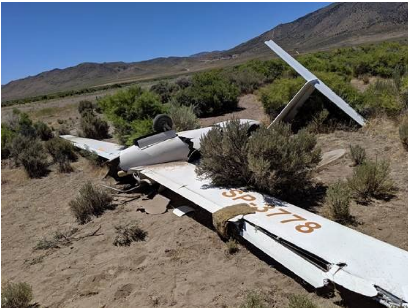
Photo 1 – View of damaged fuselage and right wing of inverted glider (Photo courtesy of tow pilot)
