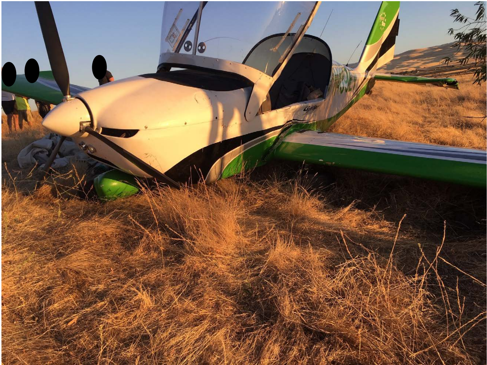
Photo 2 - View of fuselage and left wing damage (photo courtesy of the FAA)
