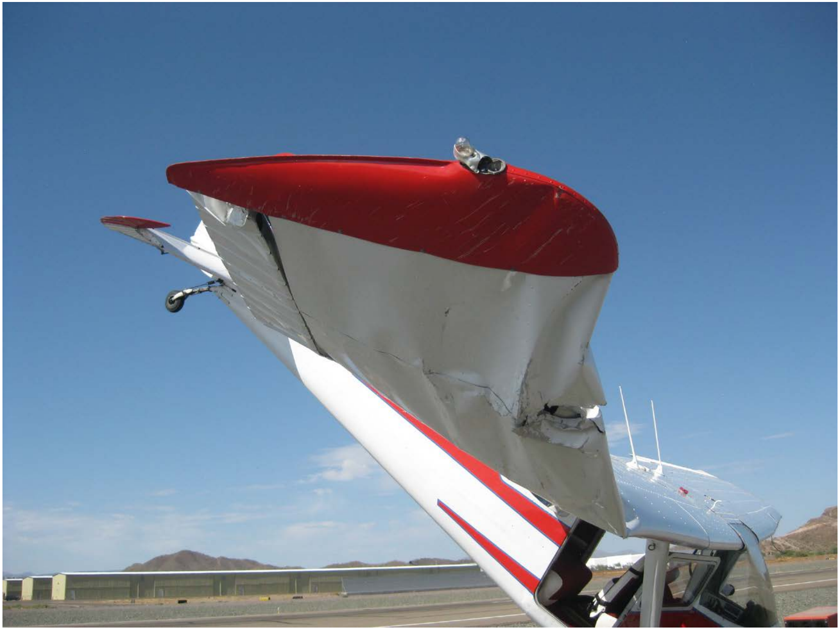
Photo 1 – View of damage to the right wing and aileron (Courtesy of FAA)
