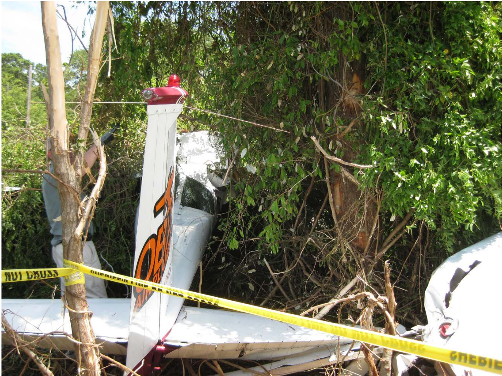
Photo 3 - View of horizontal stabilizer and elevator damage (photo courtesy of the FAA)
