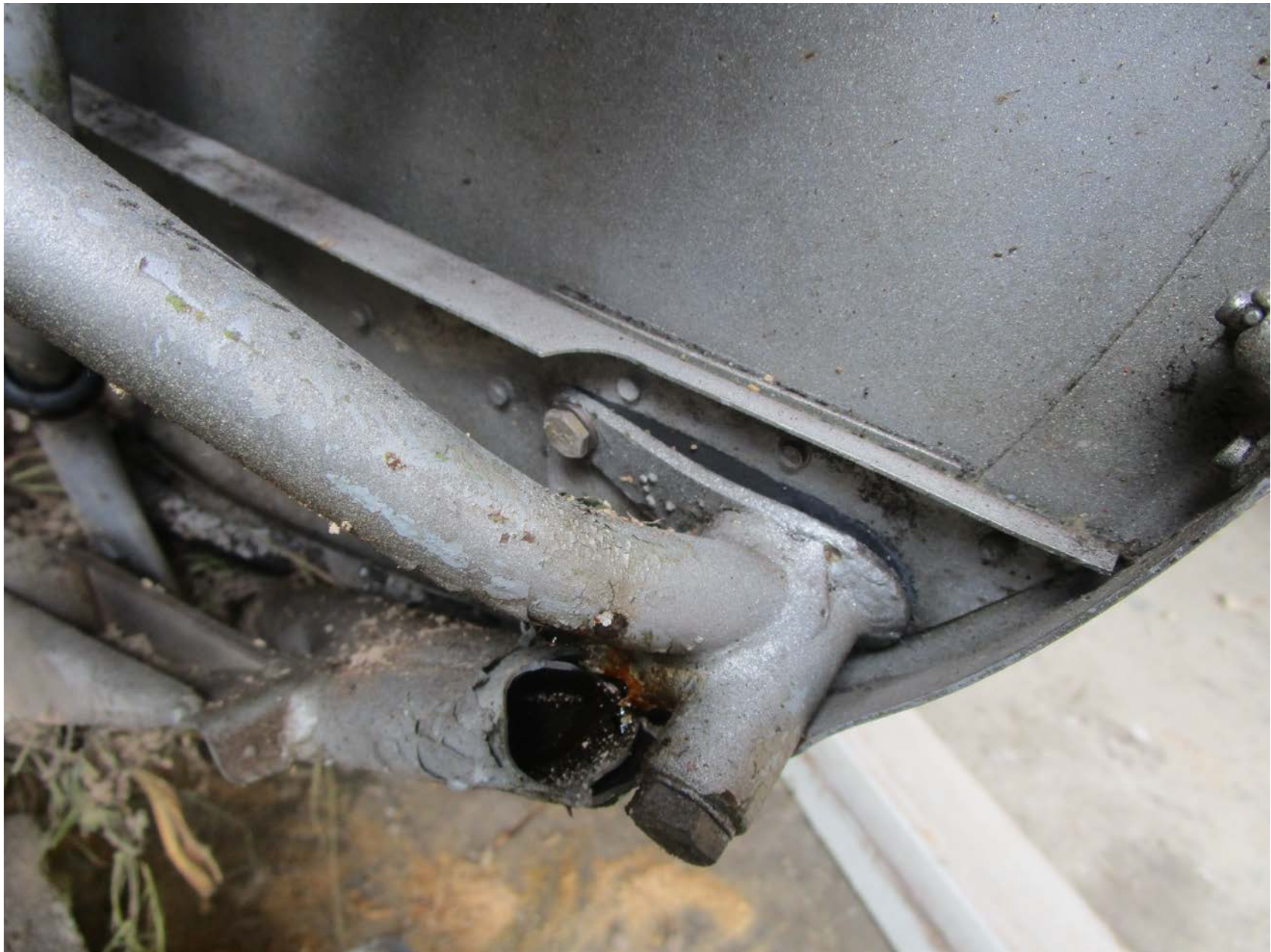
Photo 1 – View of damage to the airplane’s lower left engine mount (Courtesy of FAA)
