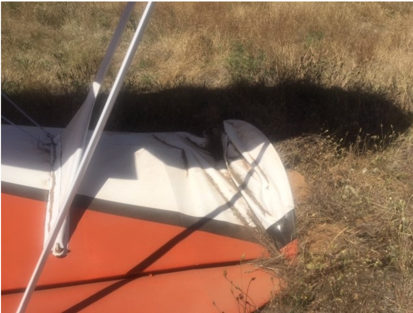
Photo 2 – View of damaged lower right wing (Photo courtesy unknown)
