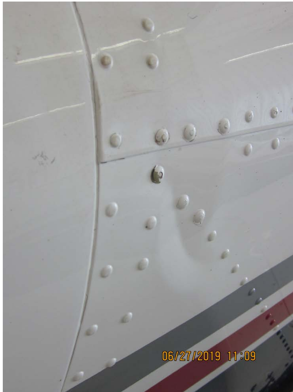
Photo 2 - View of fuselage damage (photo courtesy of the FAA)
