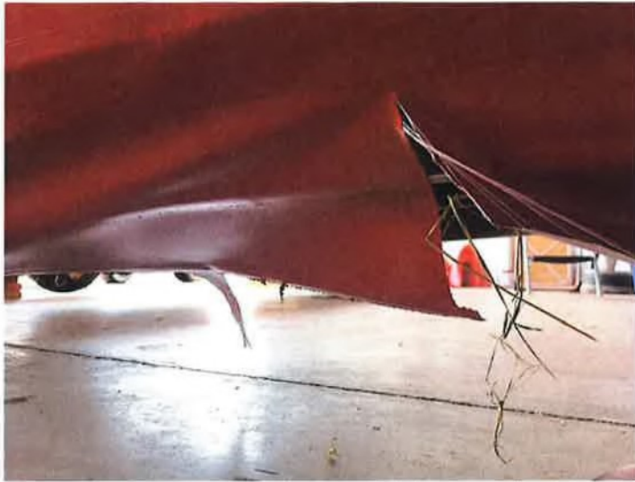
Photo taken July 2, 2019 – torn fabric on underside of fuselage.
