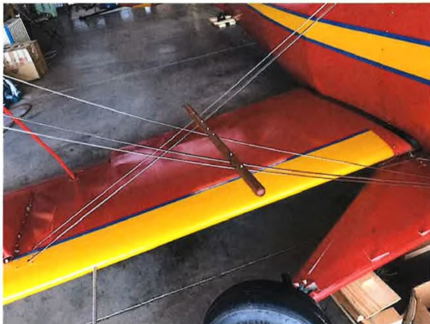
Photo taken July 2, 2019 – right wing showing slackened flying wires.
