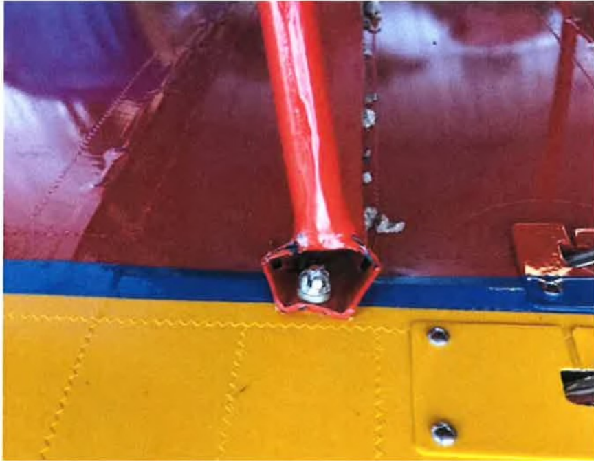
Photo taken July 2, 2019 – another view of bent end of I-strut fitting on right wing.
