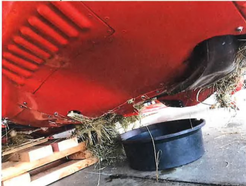
Photo taken July 2, 2019 – damaged exhaust stack and underbody from right side.
