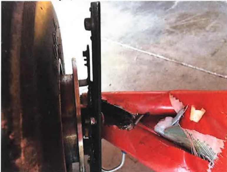
Photo taken July 2, 2019 – damage to right landing gear (detail).
