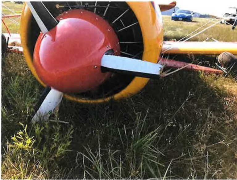
Photo taken June 30, 2019 – damaged propeller.
