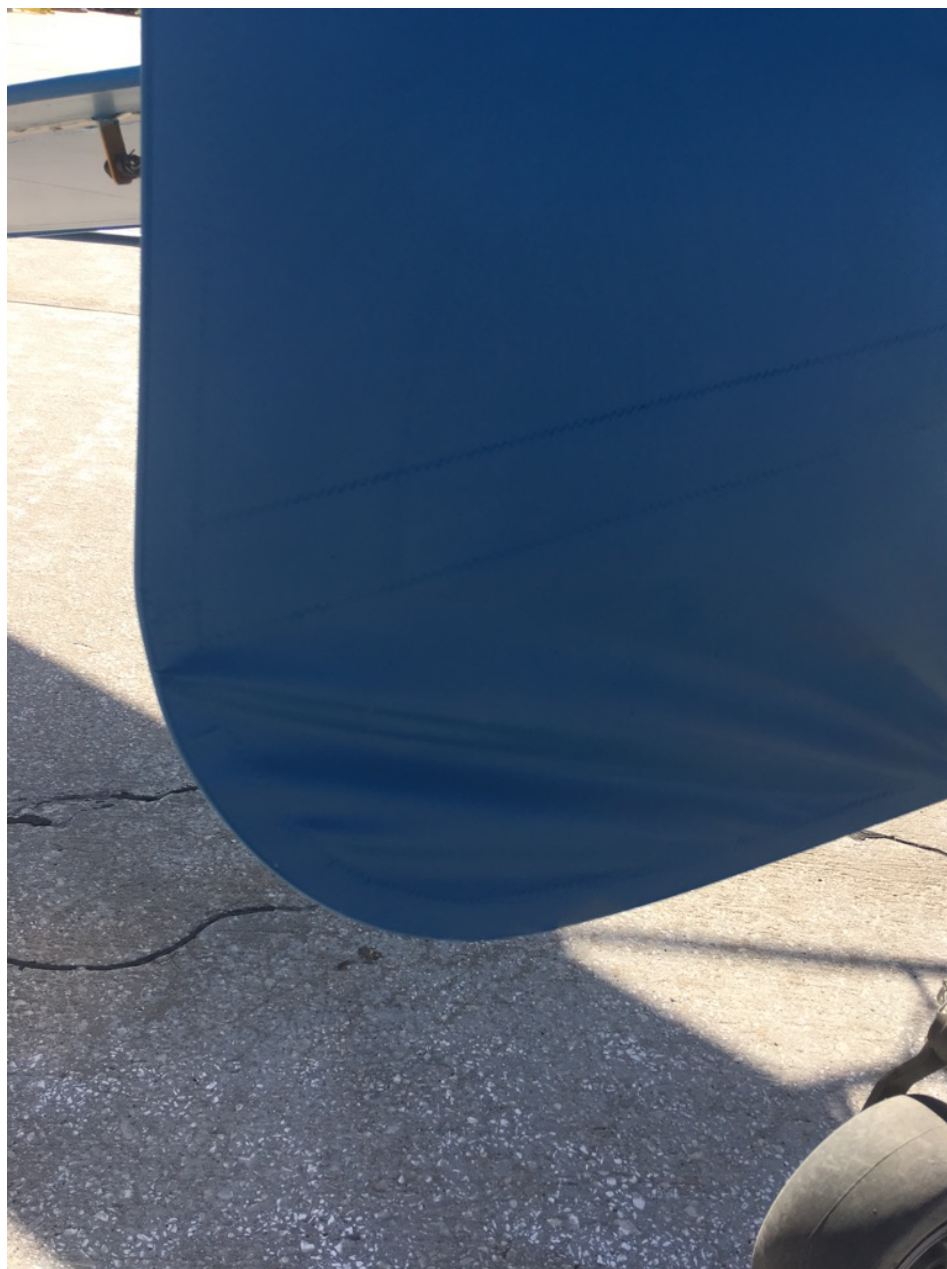
Photo 2 - View of rudder damage (photo courtesy of the pilot)
