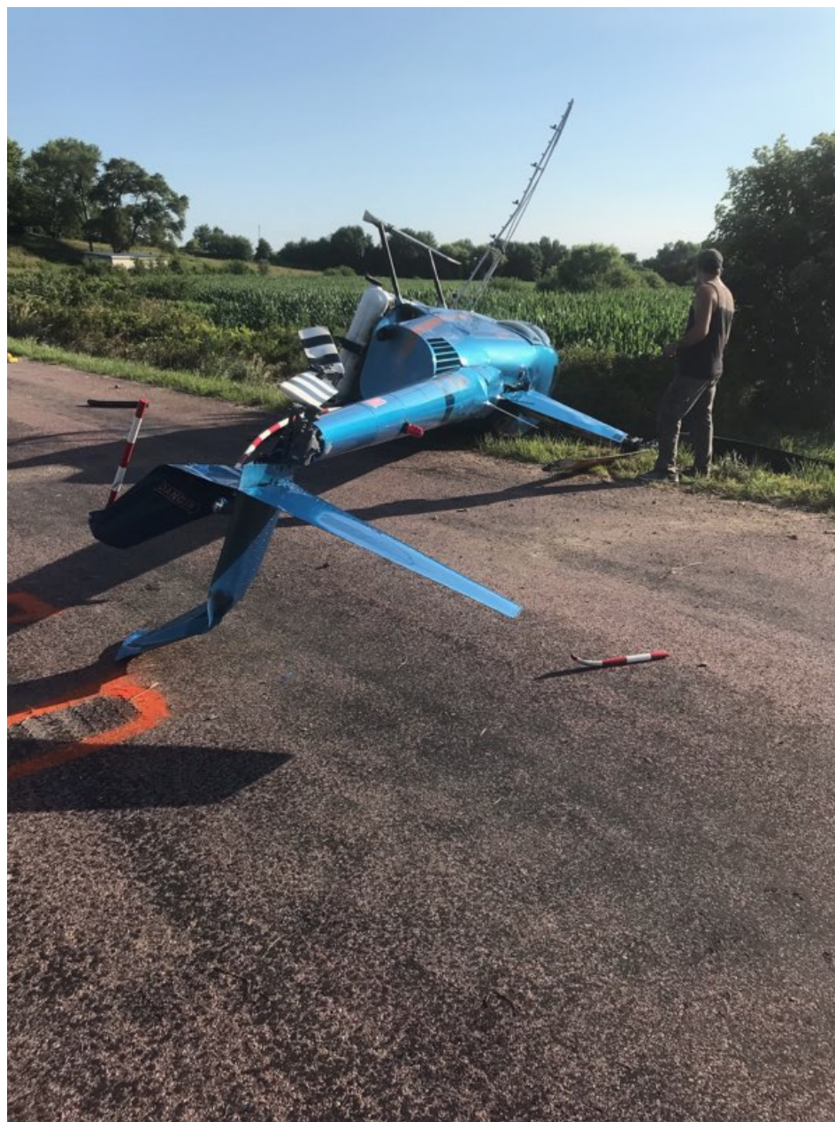
Photo – View of damage to main & tail rotor systems, empennage and fuselage (courtesy of the operator)
