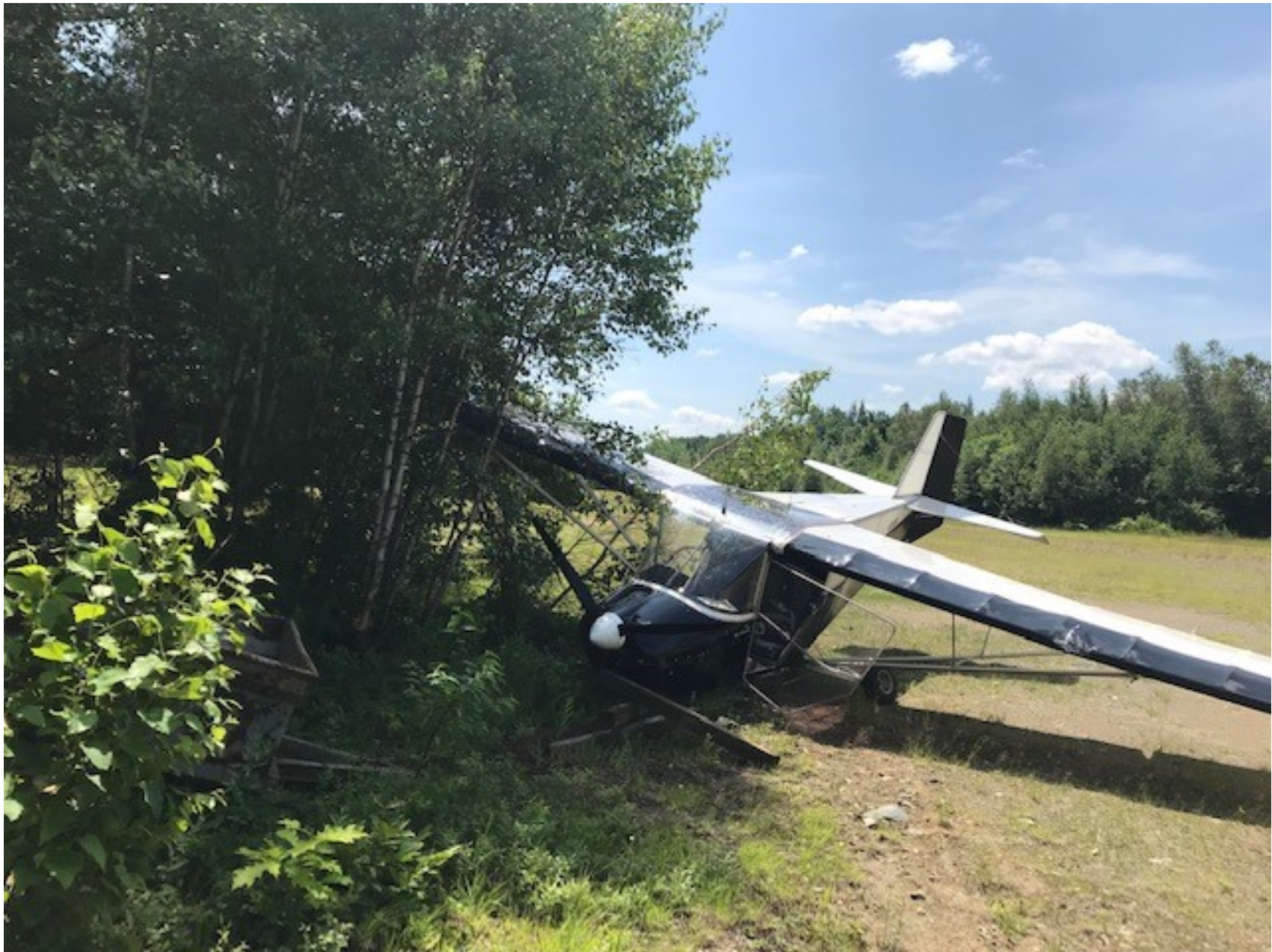
Photo 1 – View of airplane’s impact with trees and damage to lower fuselage (courtesy of the pilot)
