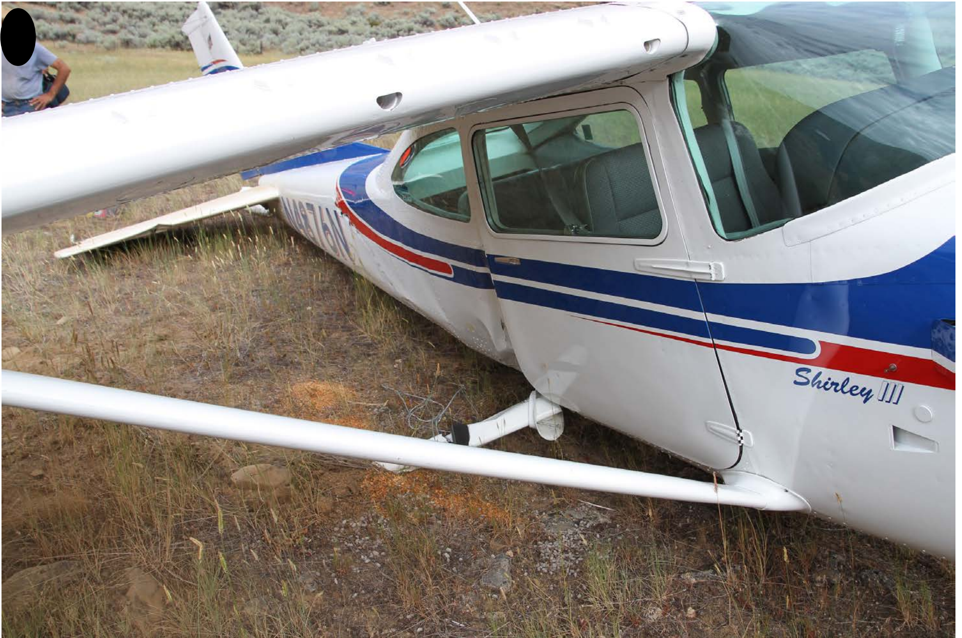
Photo 2 - View of fuselage and horizontal stabilizer damage (photo courtesy of the pilot)
