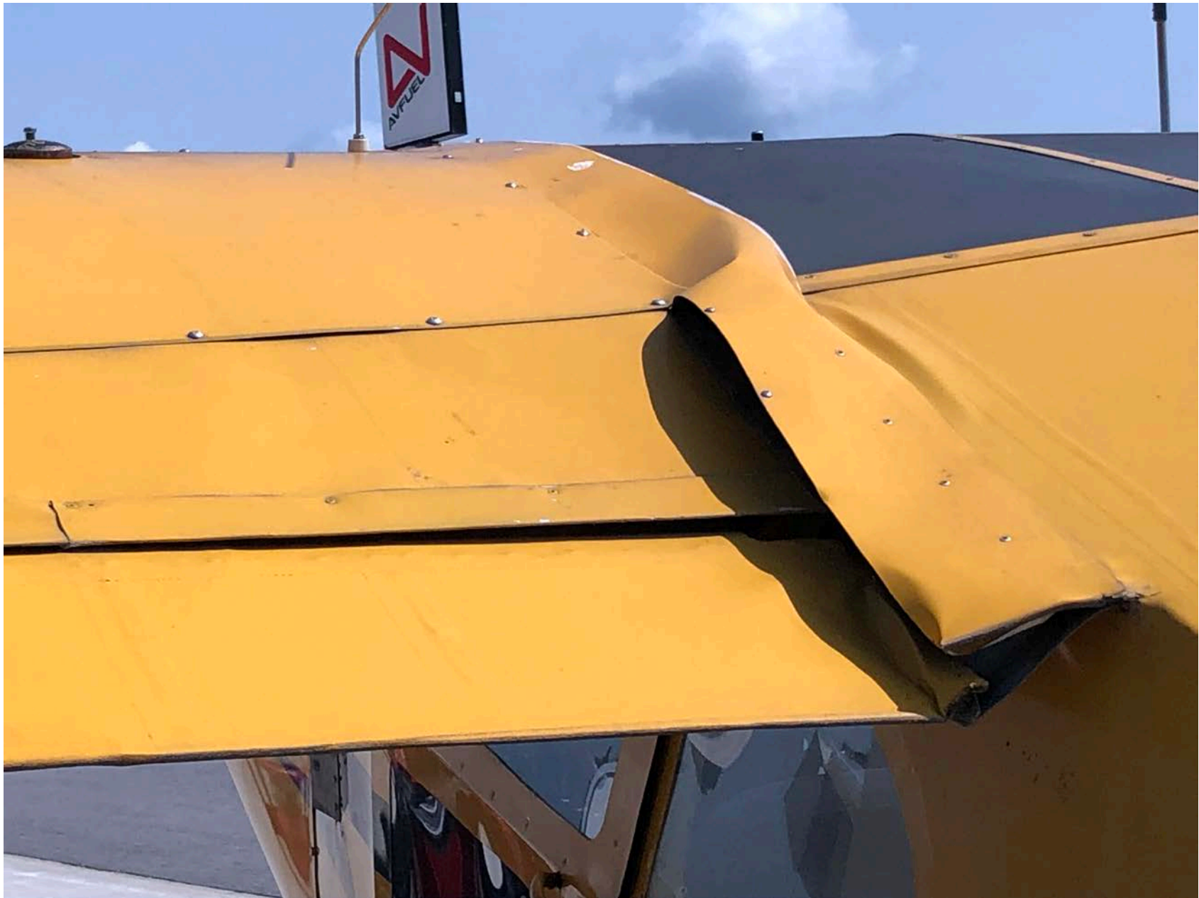
Photo 1 – View of damage to the left wing root (Courtesy of FAA)
