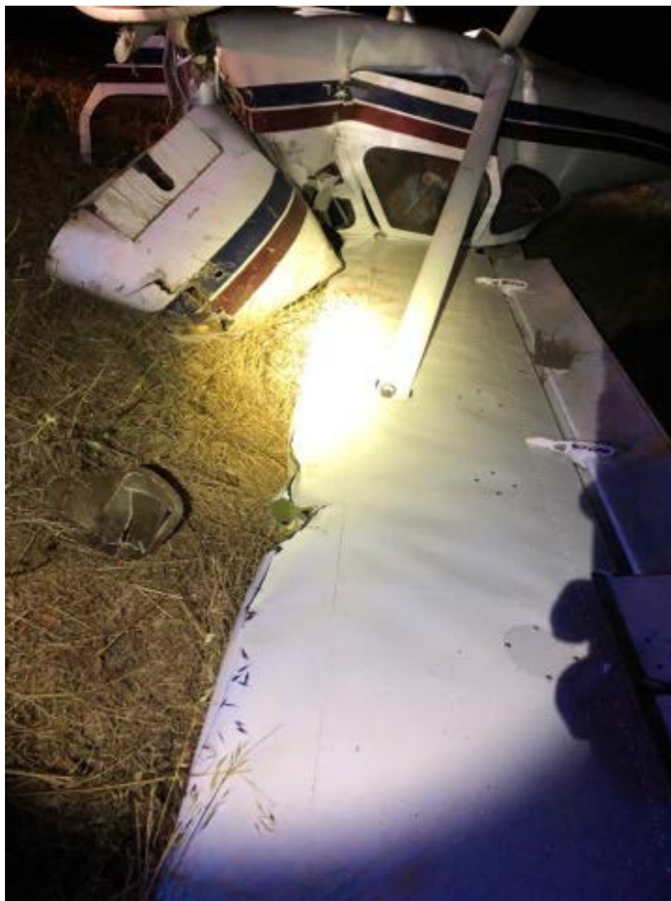
Photo 1 – View of inverted airplane with damage to the right wing (courtesy of the FAA)
