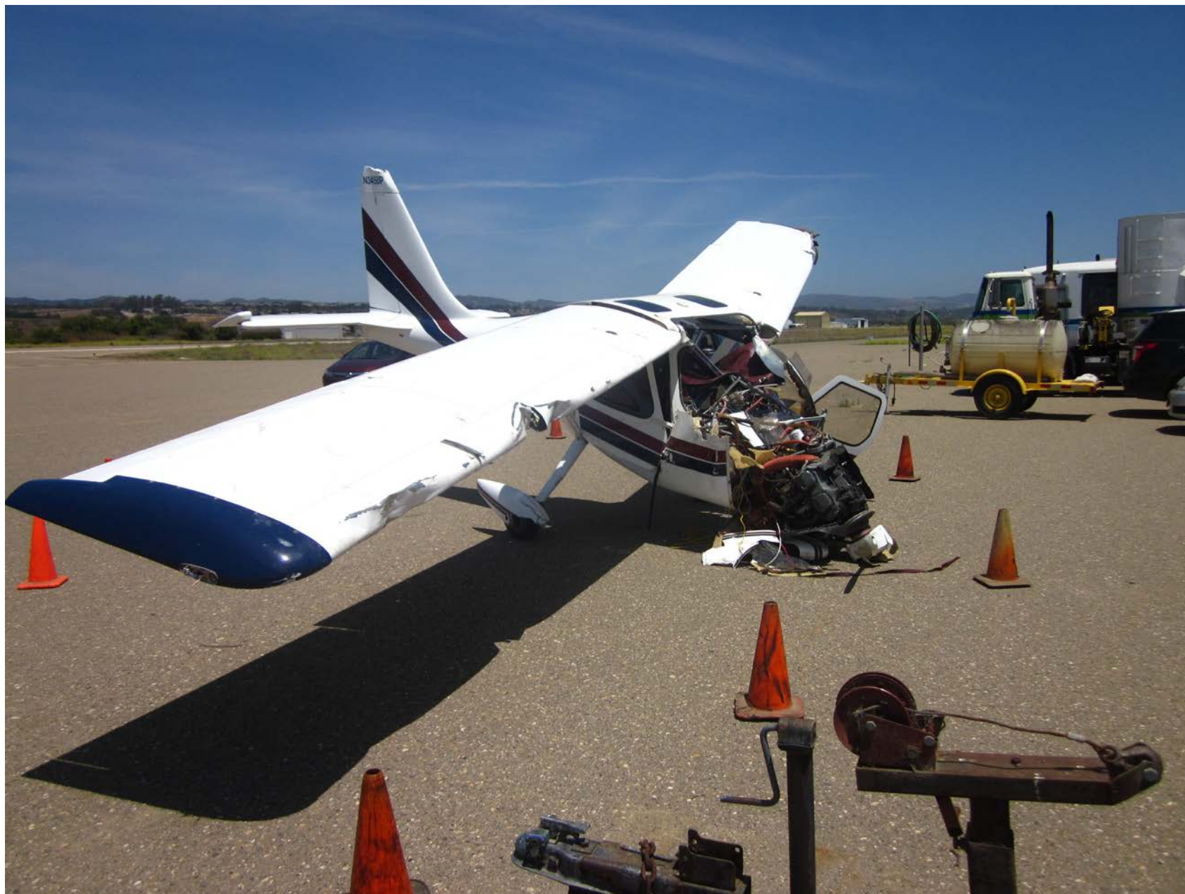
Photo 3 – View of recovered airplane with damage to both wings and fuselage (courtesy of the FAA)
