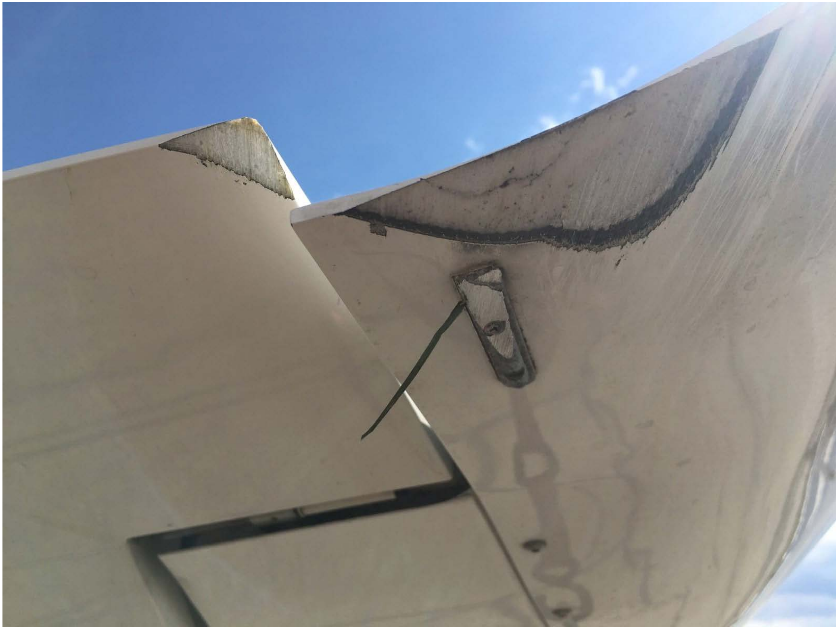
Photo 2 – View of damaged right aileron (Photo courtesy of airport operations)
