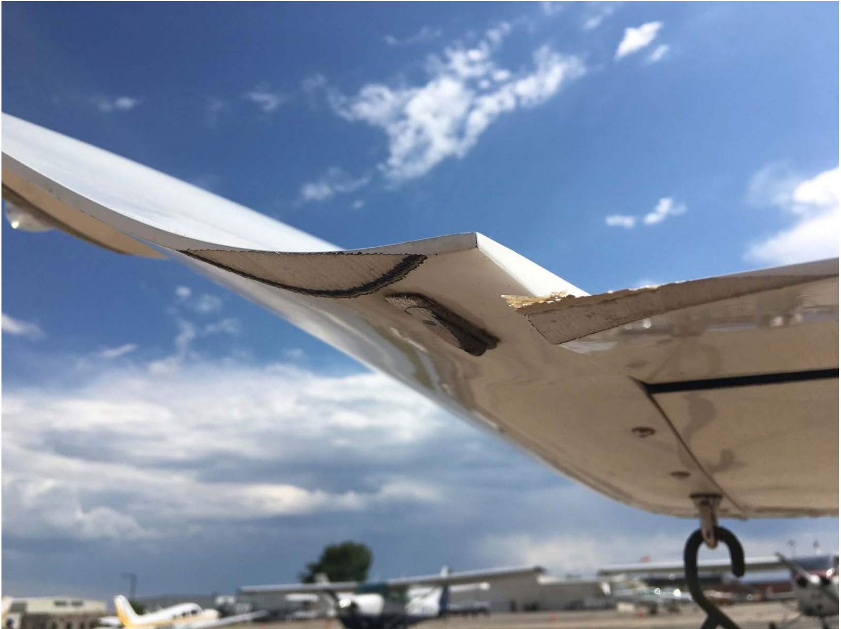
Photo 3 – View of damaged left aileron (Photo courtesy of airport operations)
