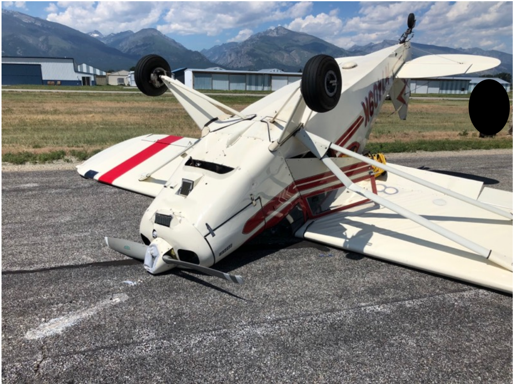
Photo 1 – View of right wing lift strut damage (photo courtesy of the FAA)
