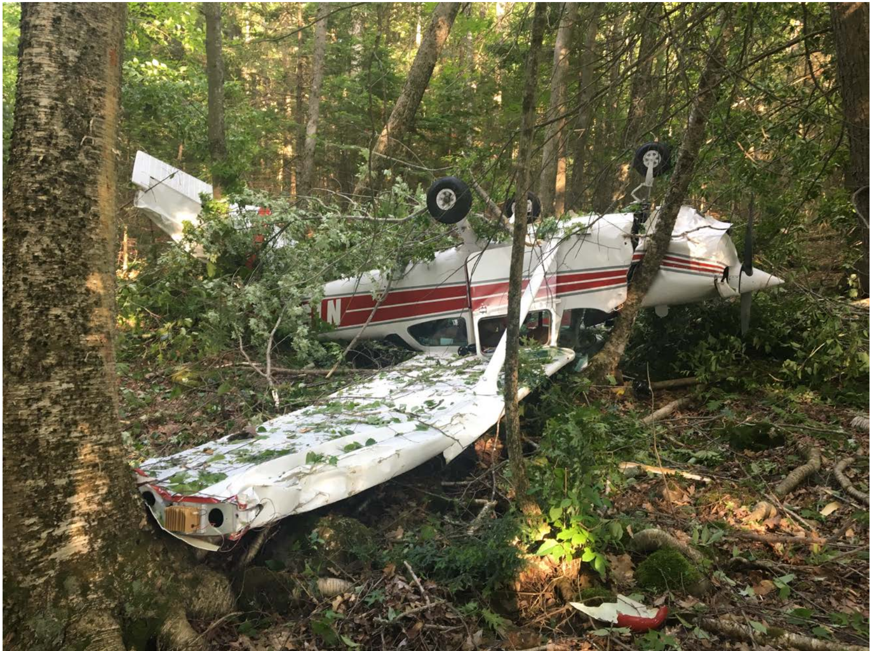
Photo 1 – View of damaged left wing and empennage (courtesy of the FAA)
